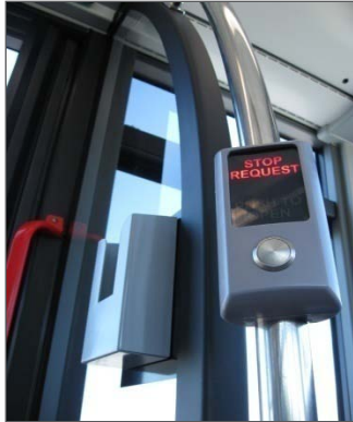
Stop request buttons at all exits and seats
