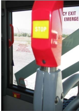
Stop request buttons at all exits and seats
