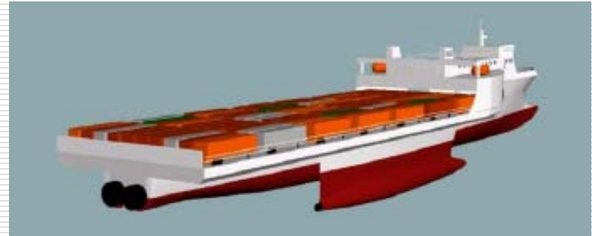
CCDoTT Trimaran 650 ft, 35 kts, 9,000 tons
