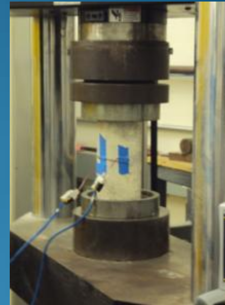
Compression tests on wrapped cylinder
