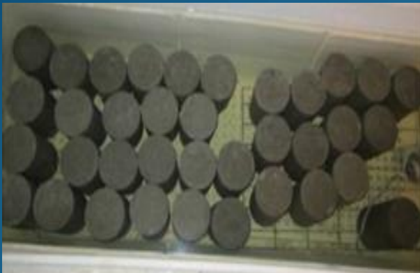
Concrete cylinders (4"x8")- 36 cylinders
