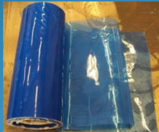
Stricture banding (Compresses & consolidates Aquawrap)
