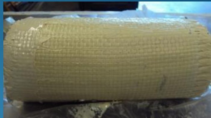
Resin impregnated & heat resistant Aquawrap 142 °C (288 °F).
