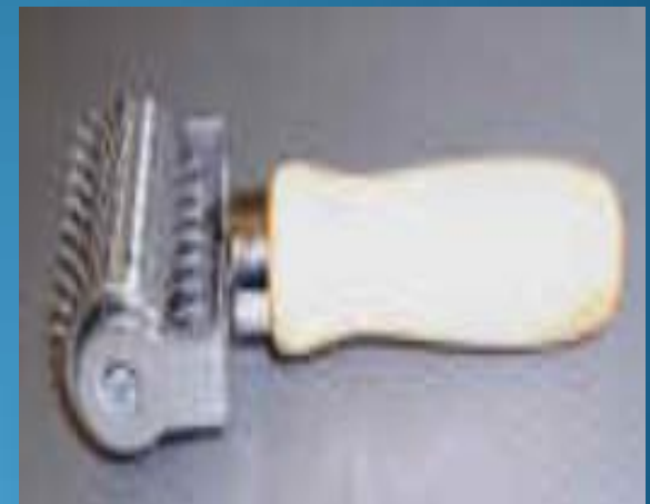
Perforator tool (Releases curing generated gas buildup)
