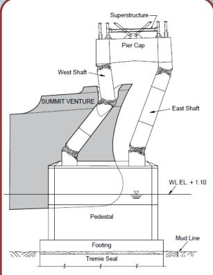
Figure C3.15.1-1—Collapse of Pier 2S of the Sunshine Skyway Bridge Subsequent to Impact by the Bow Overhang of the M/V Summit Venture
