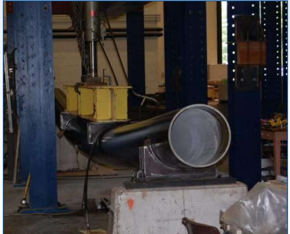
Flexural Test, WVU
