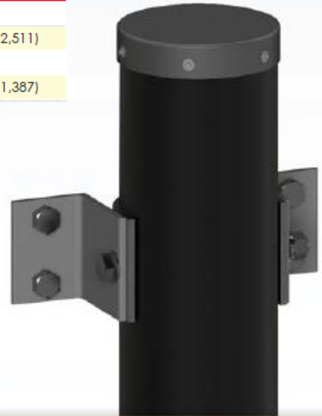
SUPERPILE Typical Dock to Pile Connection
