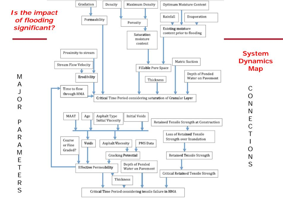
Determination of Critical Time of Flooding for Damage of Hot Mix Asphalt Pavements with Granular Base Course Layers
