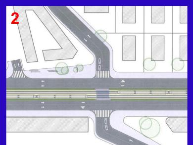
Perception: crossing zone identification Protection: green (vegetal) separator Visibility: right-angled intersection + removing obstacles Perception: LRT tracks finishing
