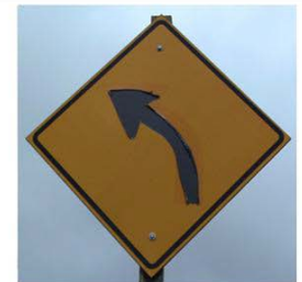
B. Peeling Damage
