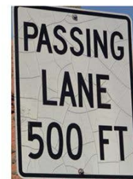
D. Cracking Damage
