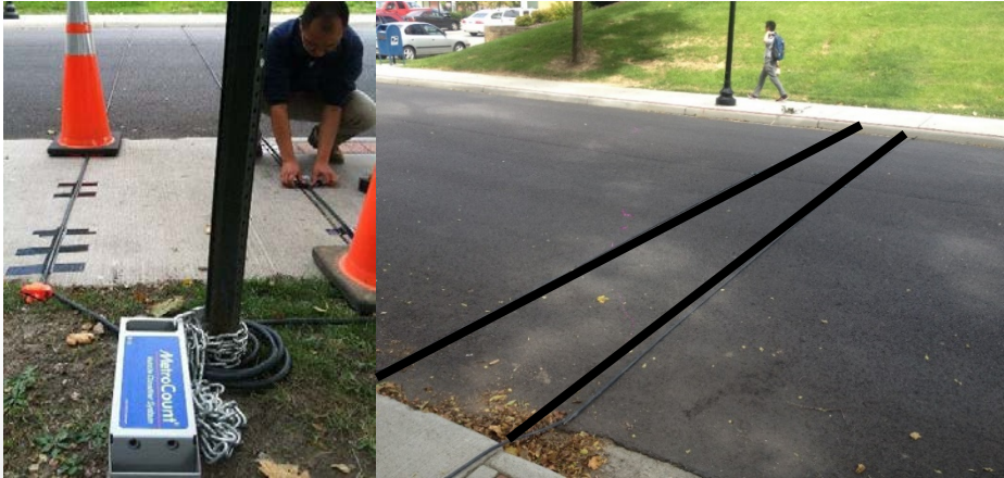
MetroCount pneumatic tube counter
