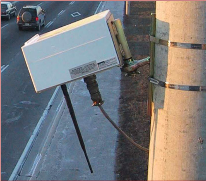
RTMS (Remote Traffic Microwave Sensor) radar
