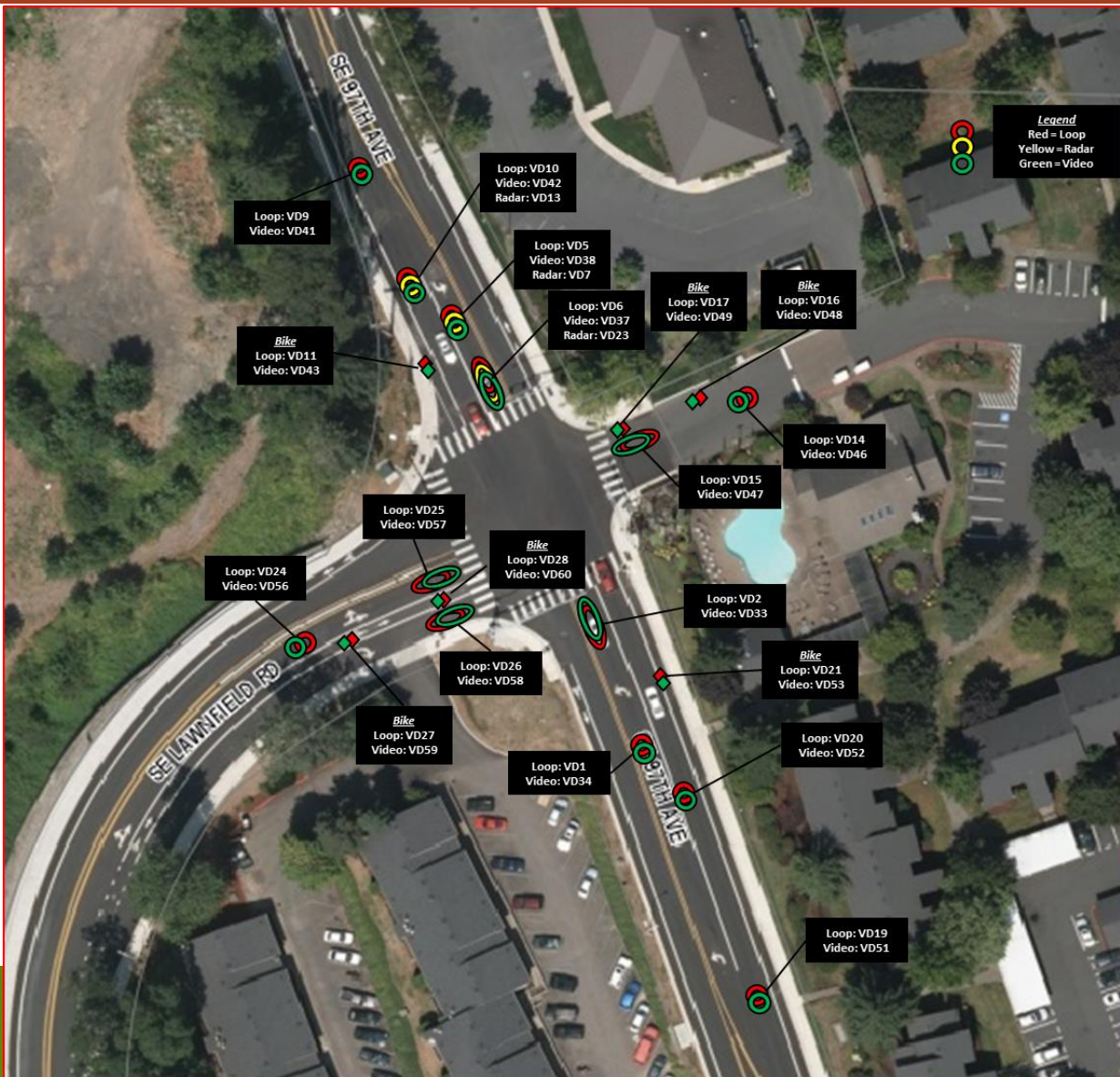
97 th & Lawnfield Road, Clackamas County
