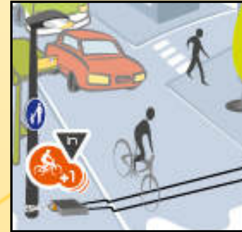
Pneumatic Tube Bicycle Counters
