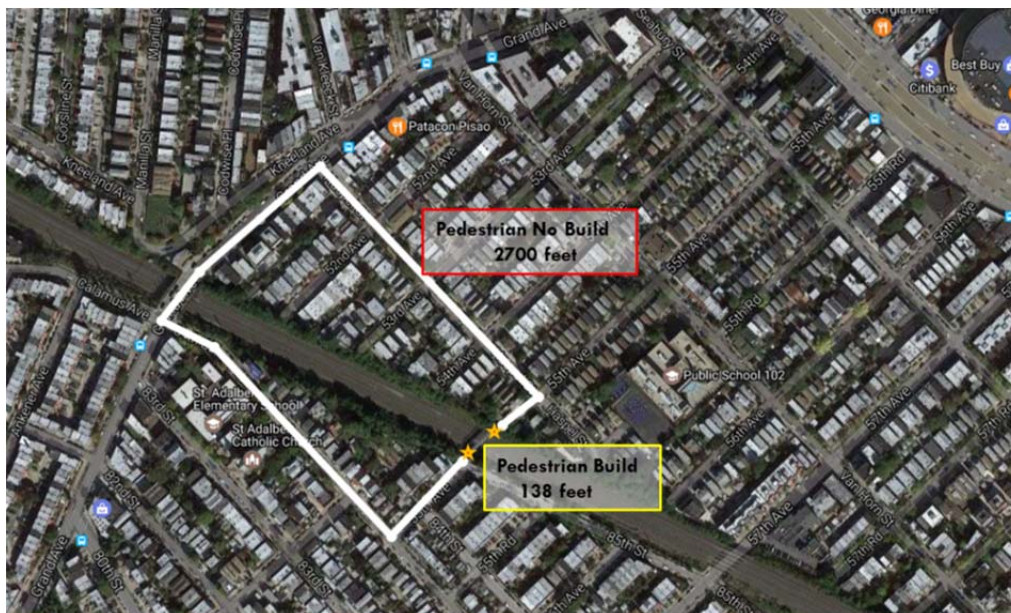
FIGURE 1 Alternate route measurement: measurement of the alternate route on the 55th Avenue pedestrian bridge.
