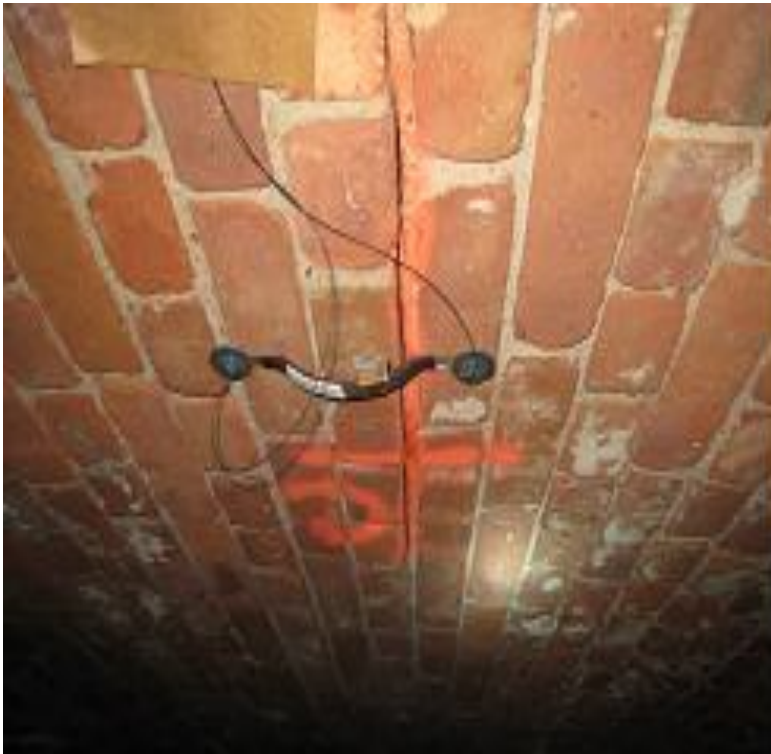
Typical FBG crack sensor (vault crown)
