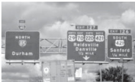
Larger route designation symbols are used for the U.S. routes to compensate for too many listings on one sign—a subject discussed in NCHRP Report 488, Additional Investigations on Driver Information Overload .
