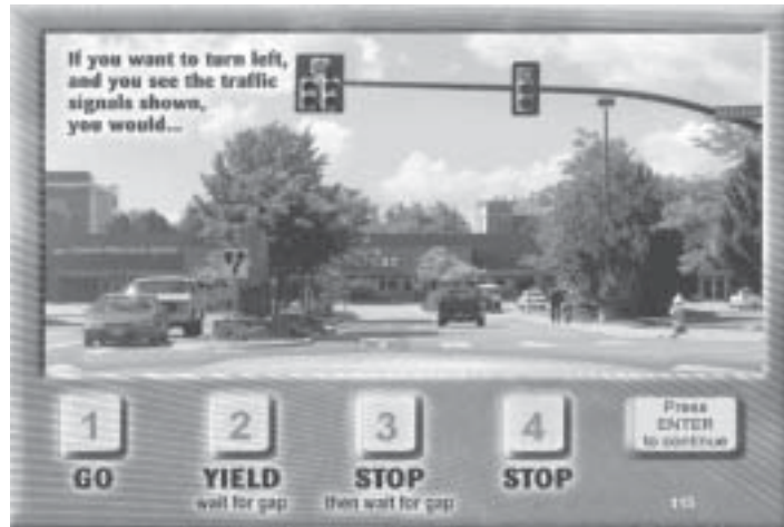
Photographic Driver Study, detailed in NCHRP Report 493, Evaluation of Traffic Signal Displays for Protected-Permissive Left-Turn Control , evaluated driver understanding of PPLT signals under various conditions.
