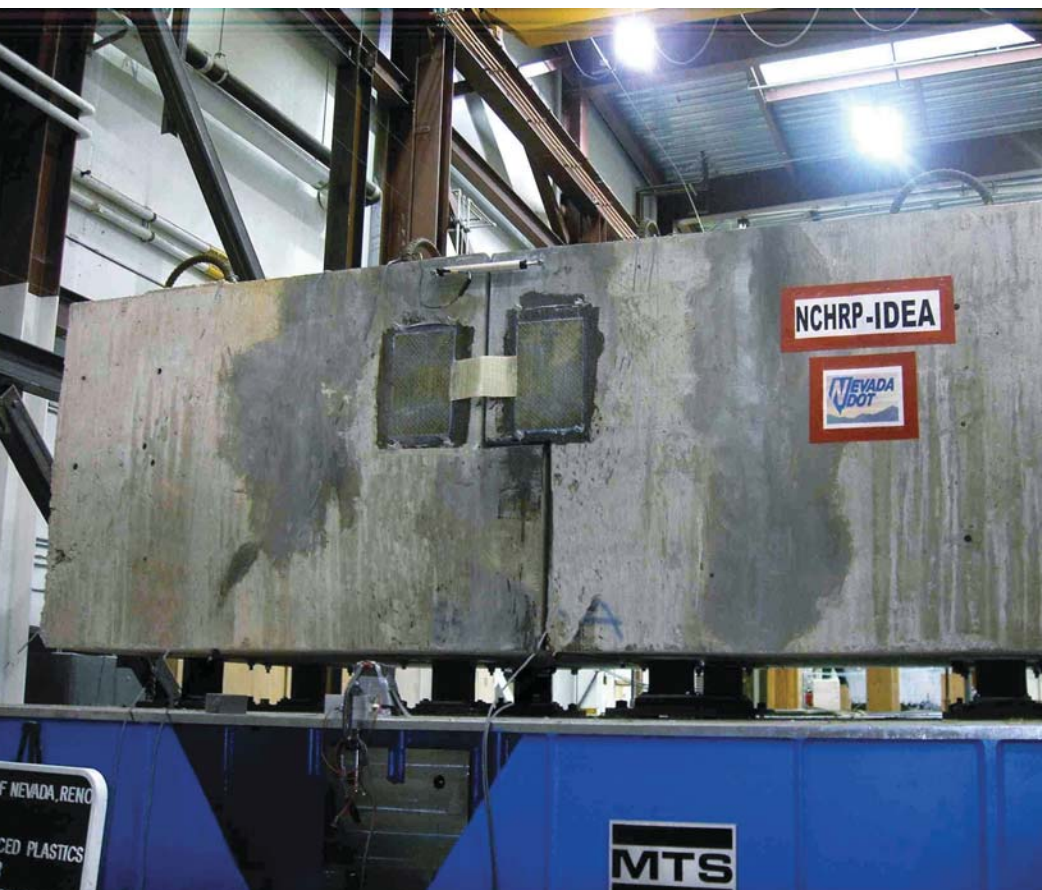
GFRP restrainer during shake table tests.
