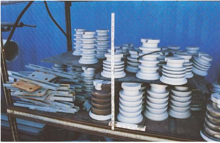
Insulators come in different shapes, sizes, and materials. Courtesy of Bay Area Rapid Transit.
