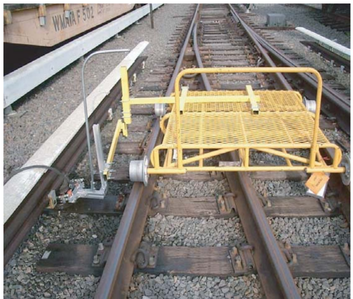
Service vehicle equipped with spray nozzle device in tests at WMATA. Testing was also conducted at the Maryland Transit Administration.
