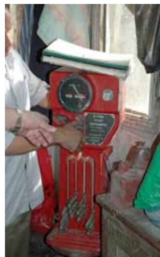
A physical token block staff machine at Qalyub, Egypt, where the August 2006 train crash occurred.
