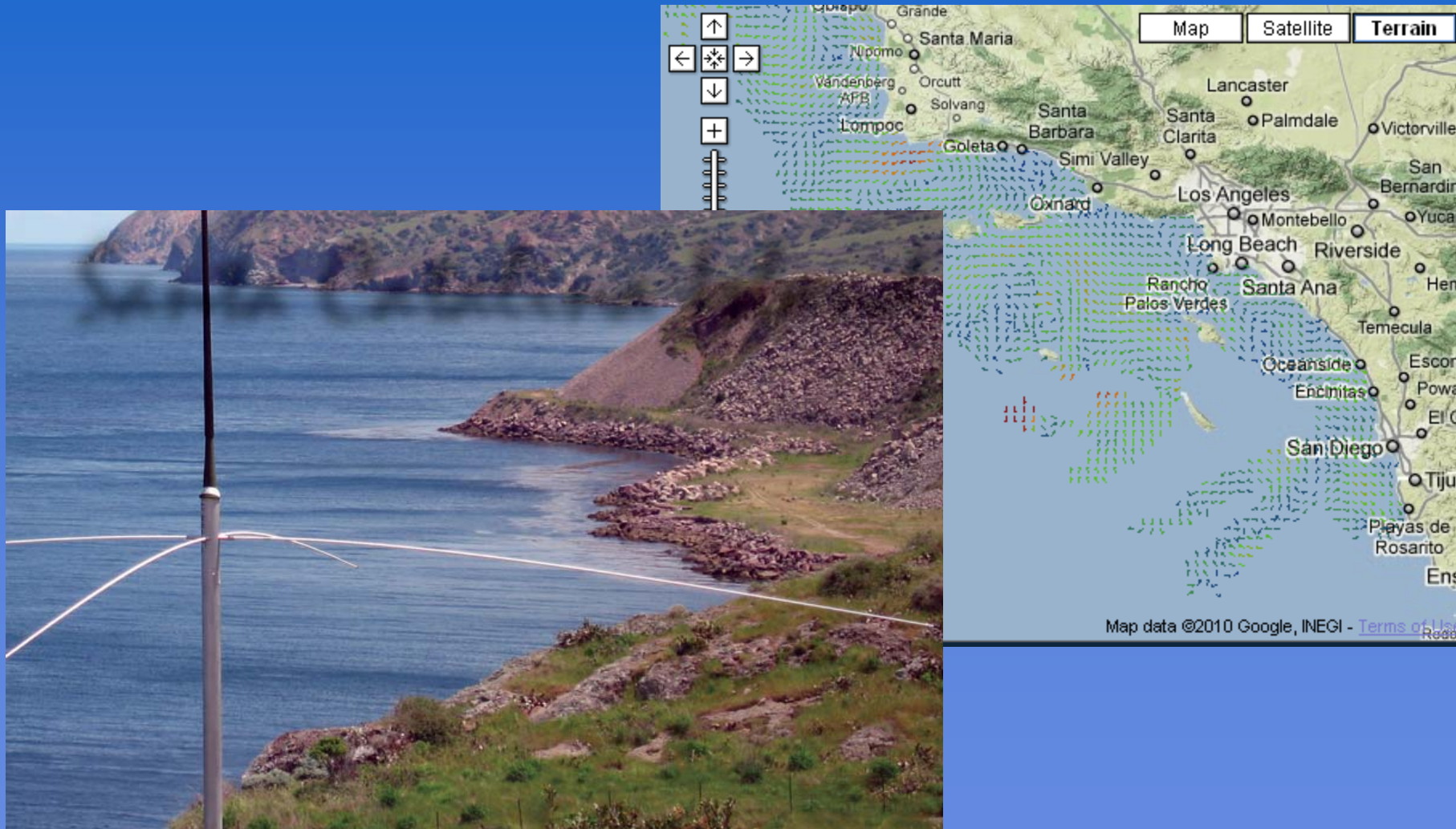
HF Radar, Santa Catalina provides surface currents
