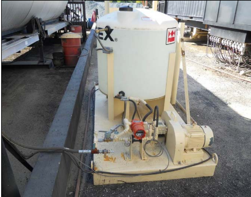
Figure 93 Terex WMA System used in Jefferson Co., FL
