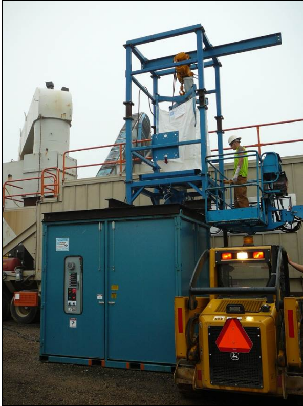
Figure 62 Advera WMA Hopper in Rapid River, MI
