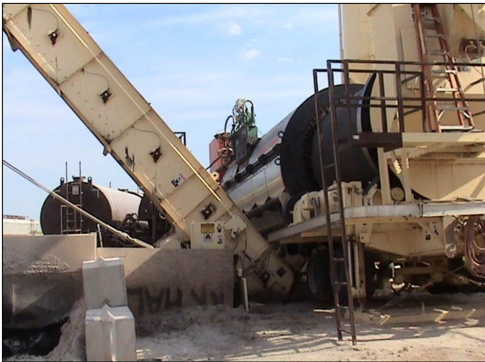
Figure 30 Drum and Point of Water Injection in Graham, TX Plant
