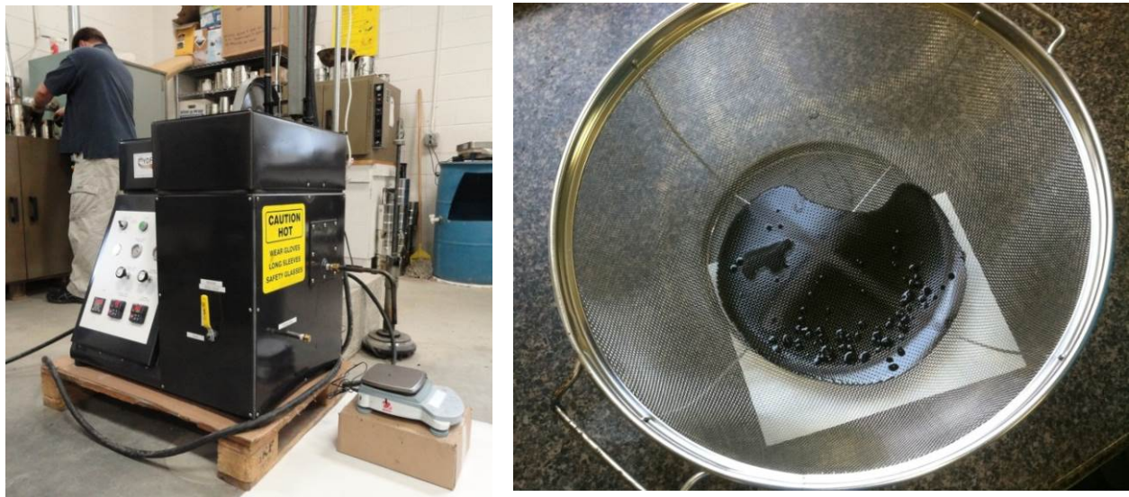
Figure 140 Hydrofoamer (left), polymer strained out of Florida PG 76-22 binder (right)
