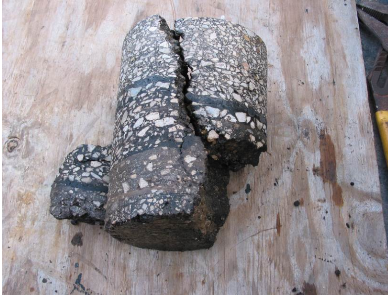
Figure 33 Photo Showing Core Taken on a Transverse Crack to demonstrate it was Reflecting from Underlying Pavement Layers
