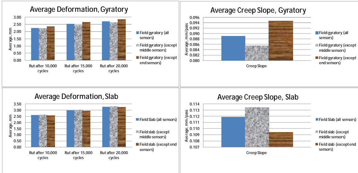
Figure 4-1-Graphical comparison of average properties of Field mixture measured using data from all measurement locations, all except three middle measurement locations, and all except two measurement locations at each end
