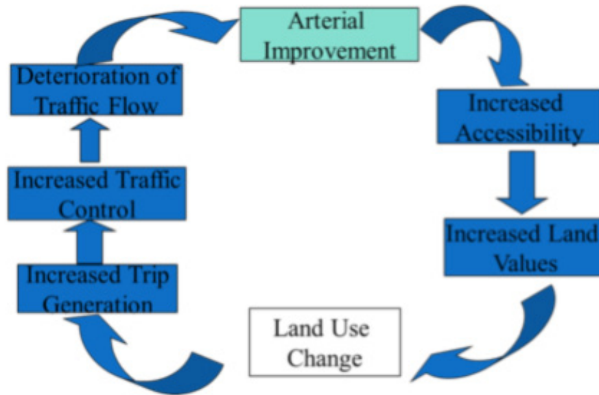
Figure 5.1 Life cycle showing the impact of land use change on transportation corridor performance (Source: GDOT)
