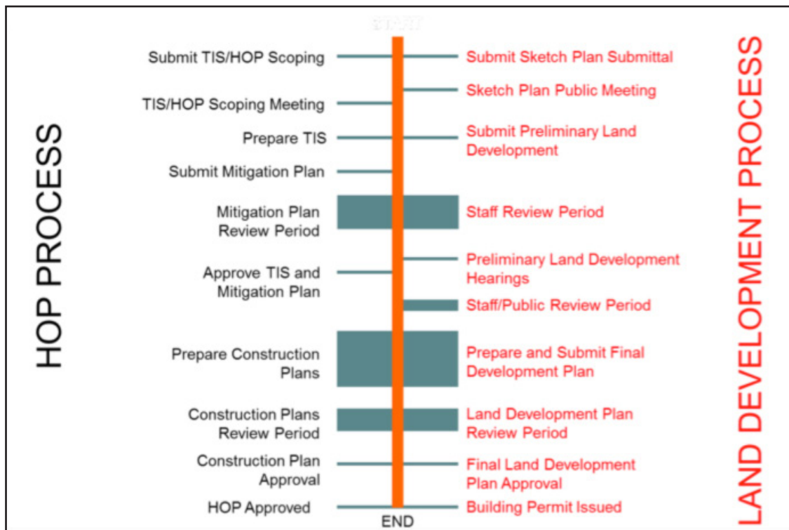
Figure 2.2 Pennsylvania land development process aligned with high-occupancy permitting process. The procedures serve as a tool to coordinate with more than 2500 municipal governments. (Source: PennDOT)
