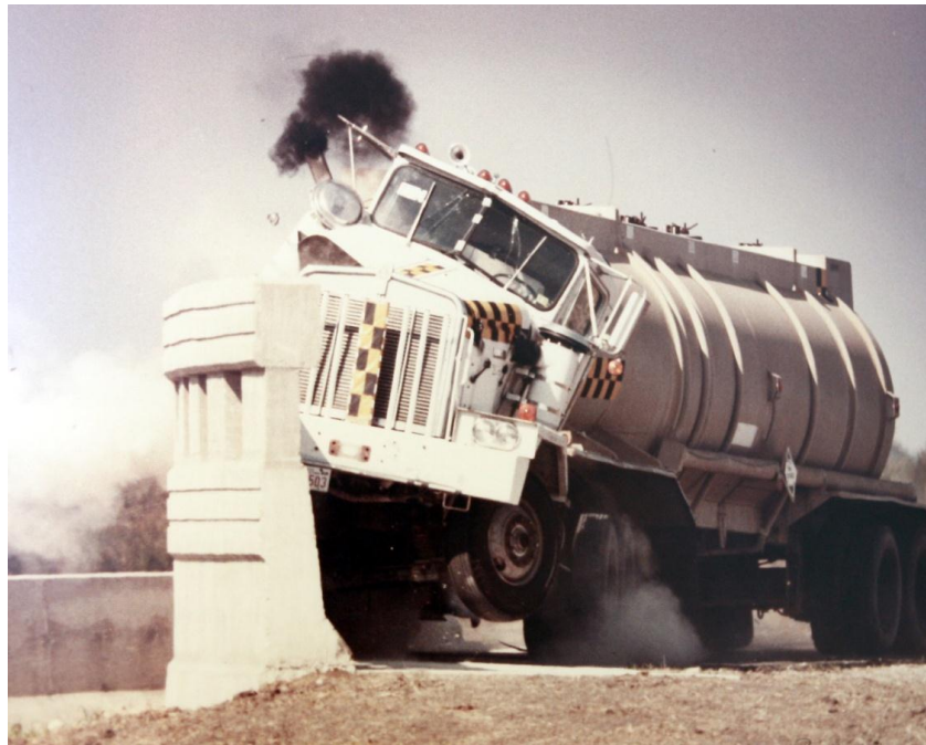
Figure 34. The only crash-tested TL6 bridge railing. [Hirsch85]
