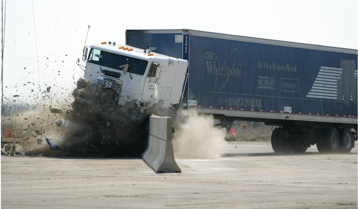
Figure 31. Tractor Trailer Truck Penetration of Concrete Median Barrier.
