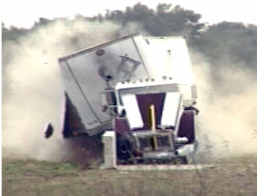
Figure 35. 50,000-lbs tractor trailer impacting a 42-inch vertical wall bridge railing. [Menges95]
