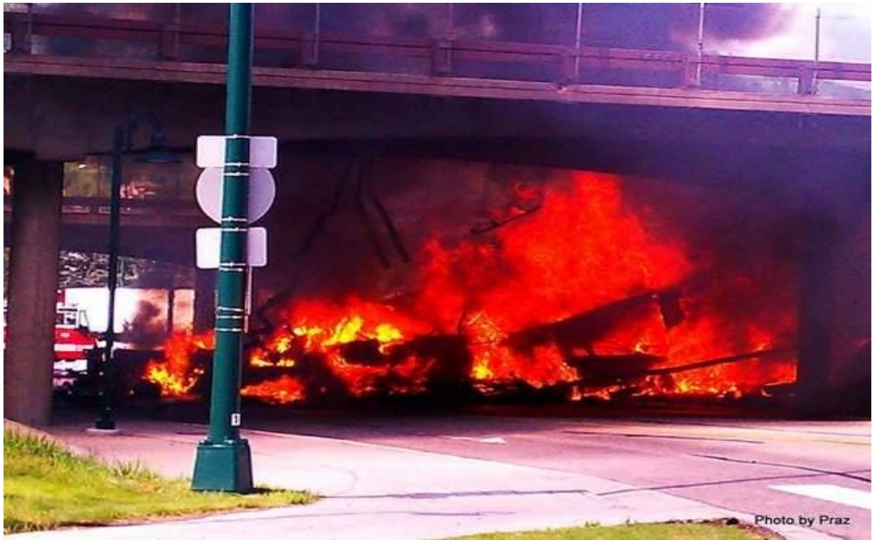
Figure 9. Truck in flames under bridge after penetrating the rail, Avon, CO. [Avon12]
