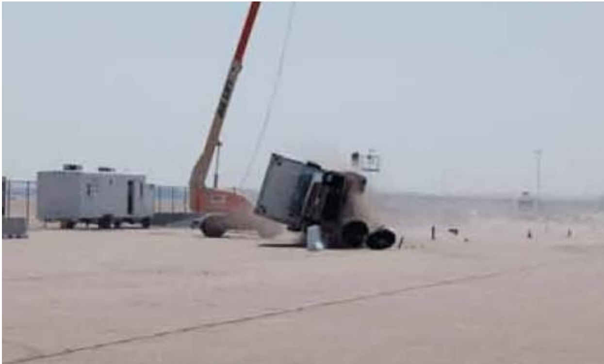
Figure 32. Single-Unit Truck Rolling Over Concrete Bridge Rail.
