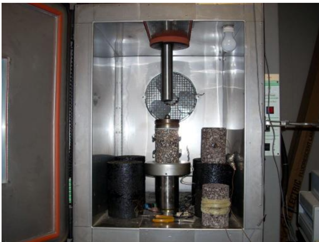
Figure 24. Photograph of Dynamic Modulus Testing Equipment.
