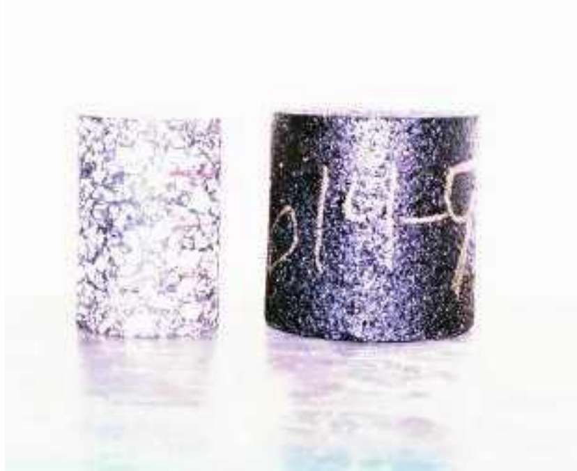
Figure 23. Final Dynamic Modulus Tests Specimen.
