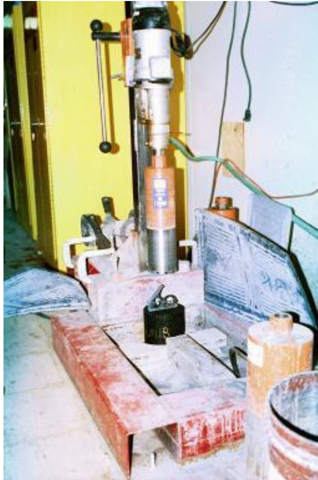
Figure 21. Portable Core Drilling Machine and Stand.
