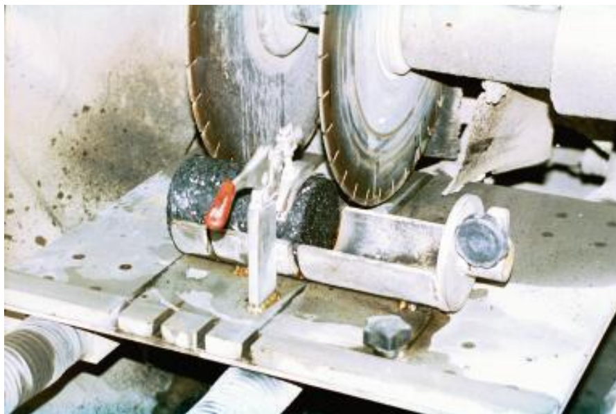
Figure 22. Double-Bladed Saw with 100-mm Core.
