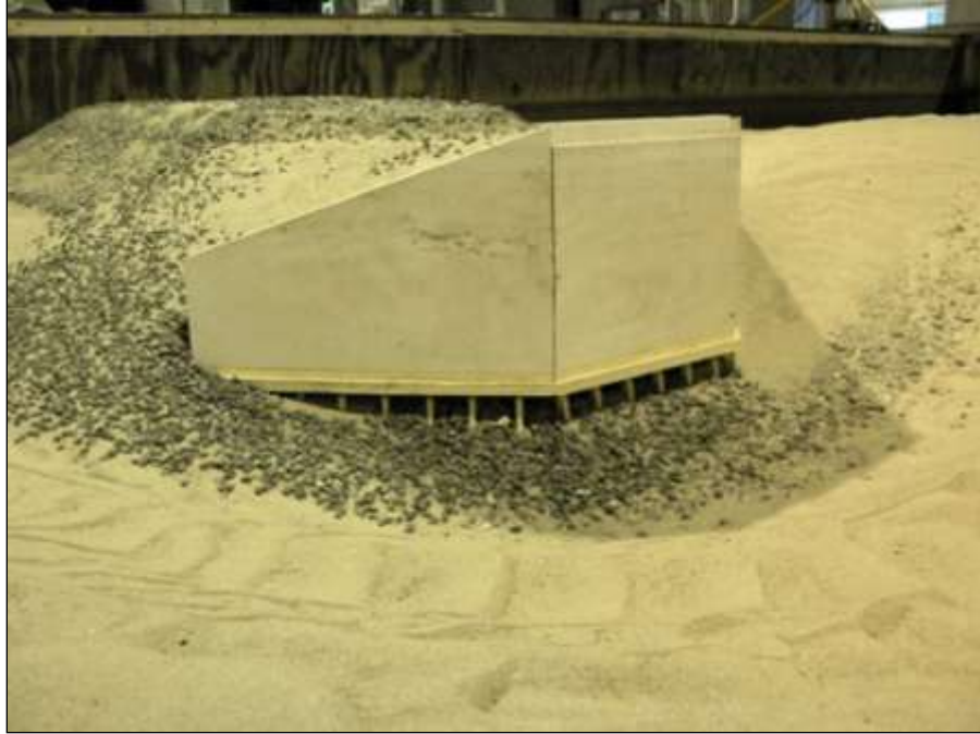
Figure 9-10. Resulting scour hole of a wing-wall abutment with L/0.5B = 0.67
