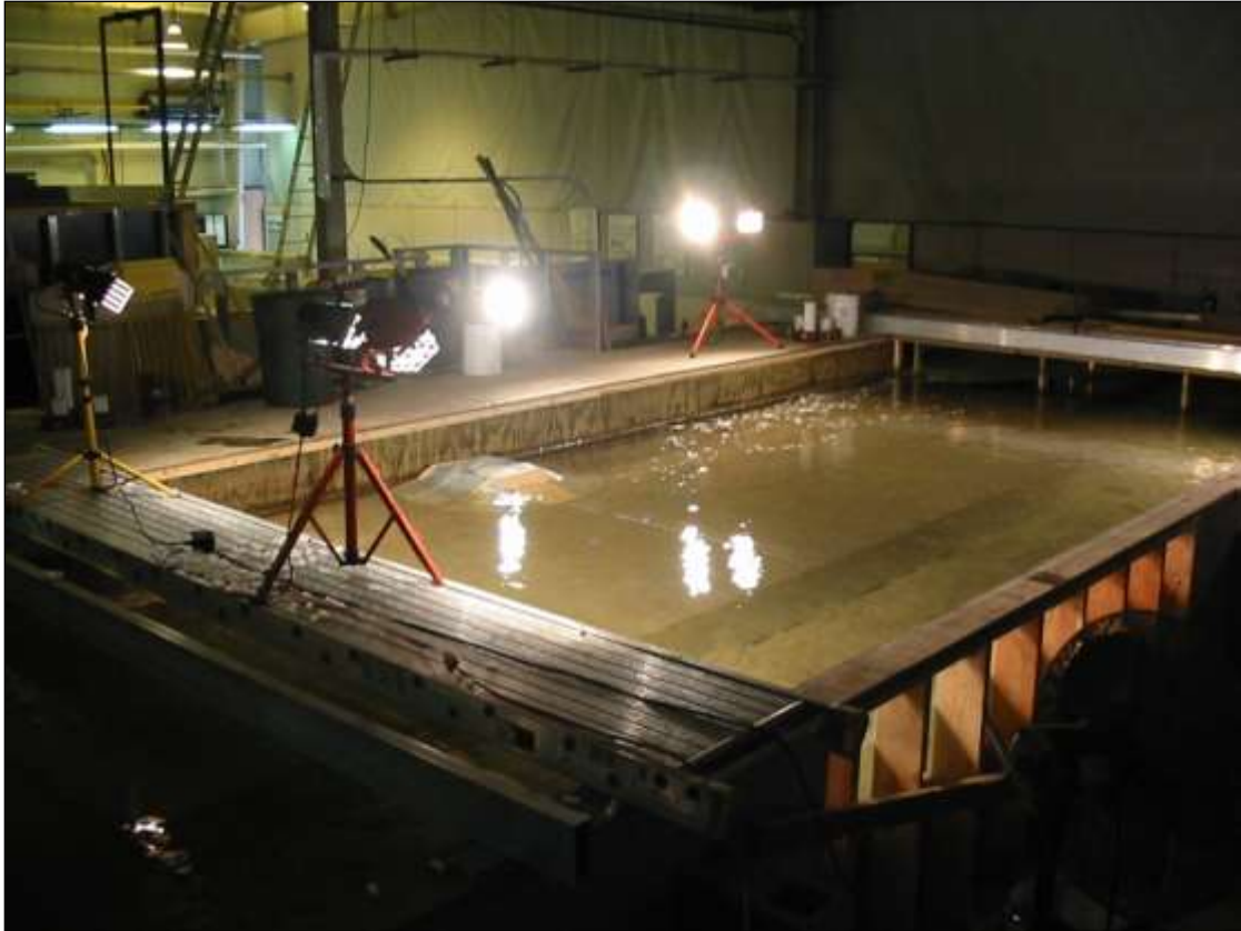
Figure 6-20. Photo showing the experimental flume and LSPIV set up
