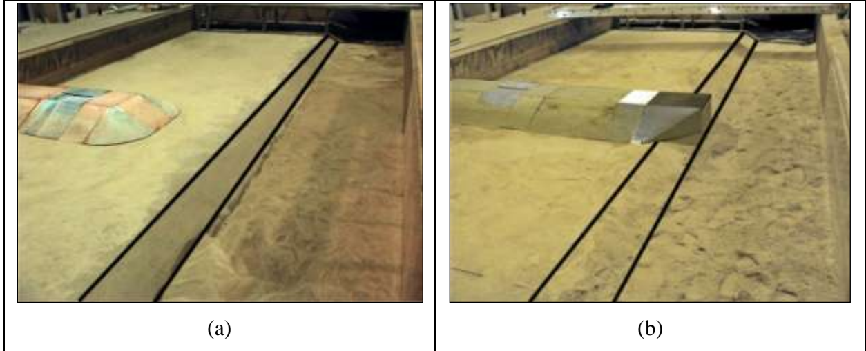
Figure 6-10. Photos showing initial set up for experiments with fixed embankment over floodplain: (a) spill-through abutment, and (b) wing-wall abutment – dark lines are drawn to indicate the sloping bank.
