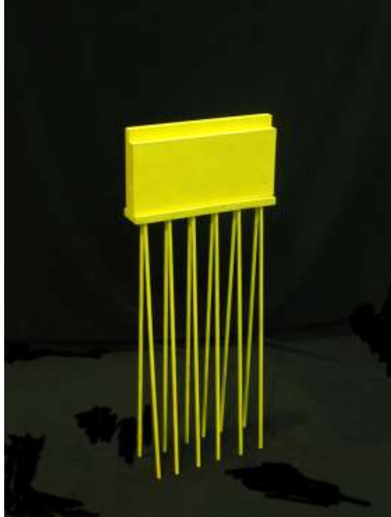
Figure 6-6. Model standard-stub column (1:30 scale)
