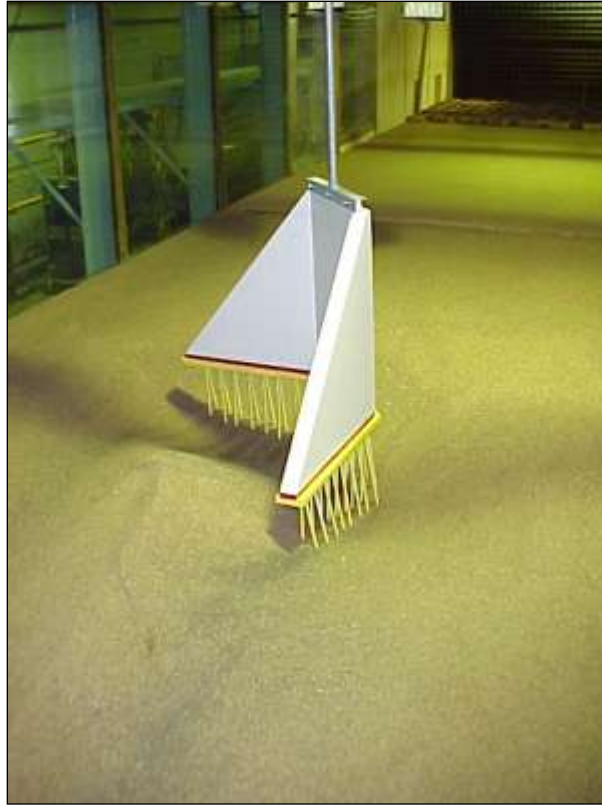
Figure 6-18. View of model of exposed wing-wall column in the flume shown in Figure 6-17
