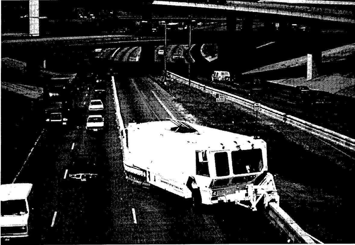
Figure 5-11. Moveable Barrier and Contraflow HOV Lane on the East R. L. Thornton Freeway in Dallas (I-30)
