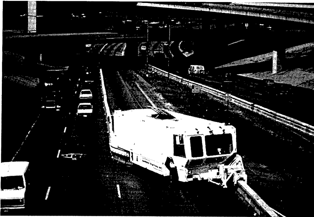
Figure 2-11. Moveable Barrier and Contraflow HOV Lane on the East R. L. Thornton Freeway in Dallas (I-30E)
