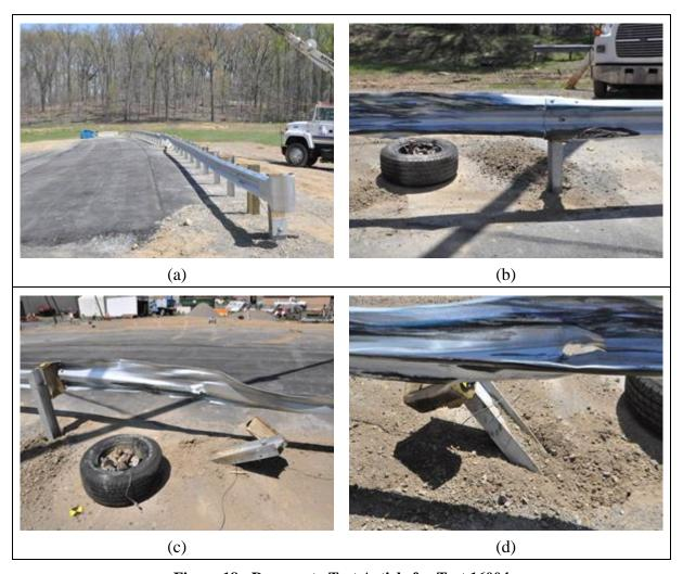
Figure 18 : Damage to Test Article for Test 16004
