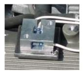
Figure 10: Typical Accelerometers and Mounting Blocks
