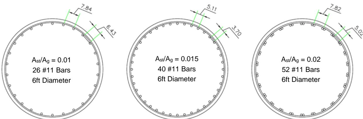
**Figure A-6. Column cross sections.**
