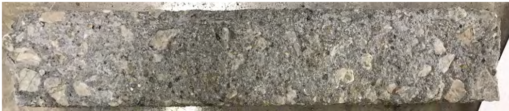
Figure G-23. Mixture 1 (M, S, N) after 56 cycles in CDF-C:FT7 testing, average visual rating 5.
