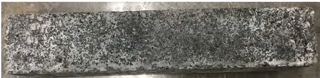
Figure G-15. Mixture 13 (M, NS, N) after 56 cycles in CDF-B:FT4 testing, average visual rating 2.
