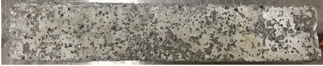
Figure G-16. Mixture 17 (M, S, S) after 56 cycles in CDF-B:FT4 testing, average visual rating 2.
