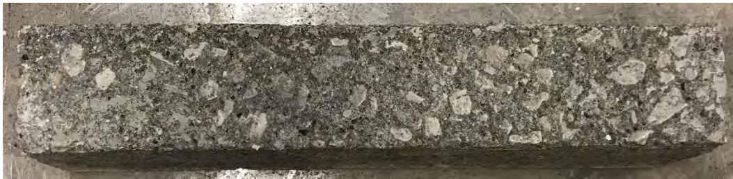
Figure G-18. Mixture 29R (M, NS, S) after 56 cycles in CDF-B:FT4 testing, average visual rating 5.
