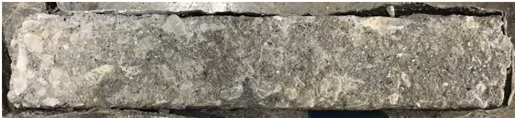
Figure G-14. Mixture 1 (M, S, N) after 56 cycles in CDF-B:FT4 testing, average visual rating 4–5.
