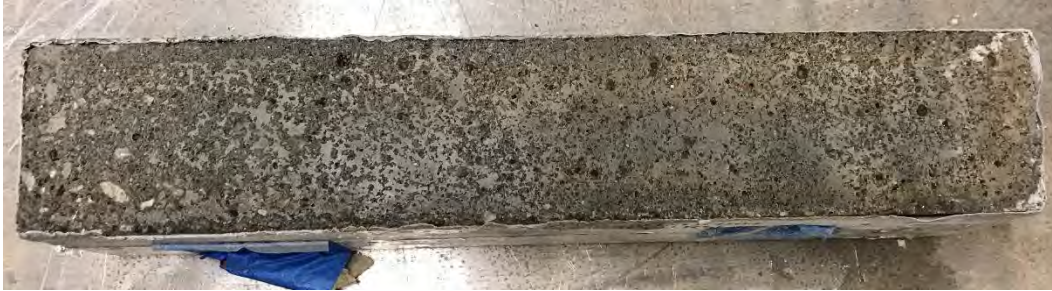
Figure G-7. Mixture 17 after 56 cycles in CDF-A:FT1 testing, average visual rating 1.
