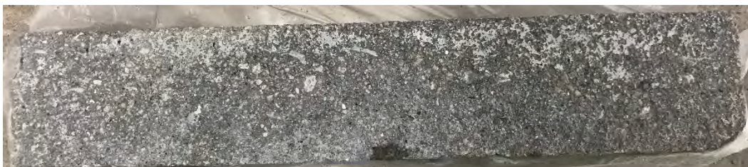
Figure G-24. Mixture 13 (M, NS, N) after 56 cycles in CDF-C:FT7 testing, average visual rating 2.
