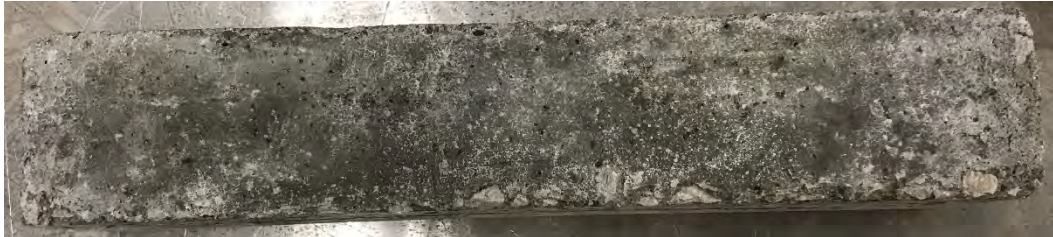
Figure G-17. Mixture 29 (M, NS, S) after 56 cycles in CDF-B:FT4 testing, average visual rating 1.
