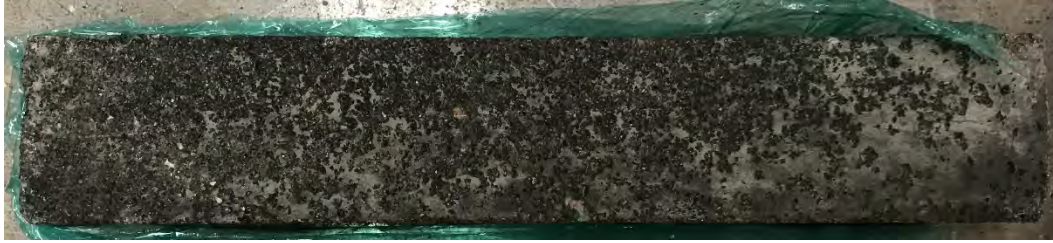
Figure G-21. Mixture 2 (A, S, N) after 56 cycles in CDF-C:FT7 testing, average visual rating 2.
