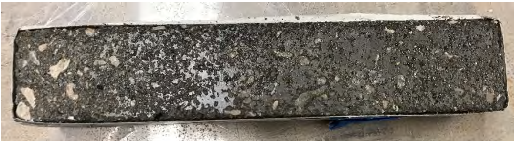
Figure G-9. Mixture 29RT after 56 cycles in CDF-A:FT1 testing, average visual rating 3.
