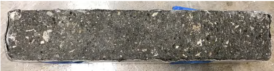
Figure G-5. Mixture 1 after 56 cycles in CDF-A:FT1 testing, average visual rating 4.
