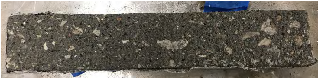
Figure G-8. Mixture 29 after 56 cycles in CDF-A:FT1 testing, average visual rating 4.
