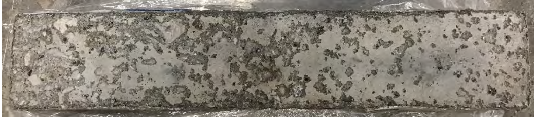
Figure G-12. Mixture 2 (A, S, N) after 56 cycles in CDF-B:FT4 testing, average visual rating 2.
