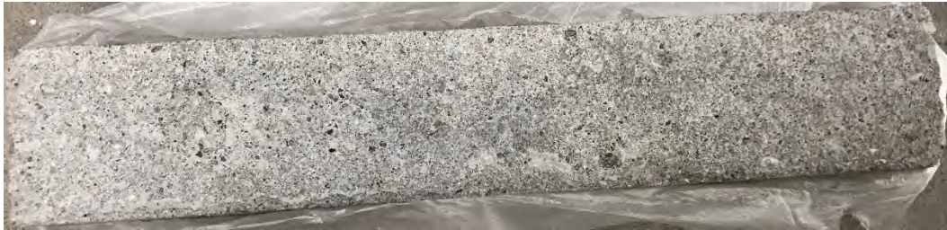
Figure G-26. Mixture 29 (M, NS, S) after 56 cycles in CDF-C:FT7 testing, average visual rating 2.
