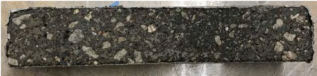
Figure G-4. Mixture 14 after 56 cycles in CDF-A:FT1 testing, average visual rating 5.
