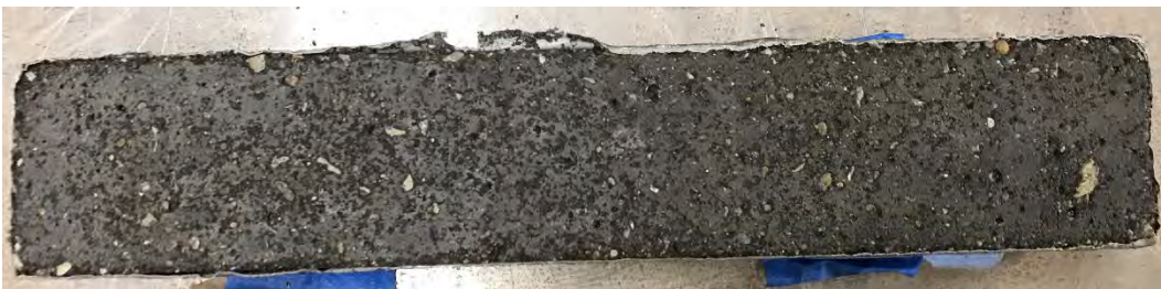
Figure G-6. Mixture 13 after 56 cycles in CDF-A:FT1 testing, average visual rating 1–2.
