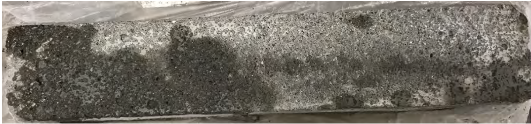
Figure G-22. Mixture 14 (A, NS, N) after 56 cycles in CDF-C:FT7 testing, average visual rating 1.
