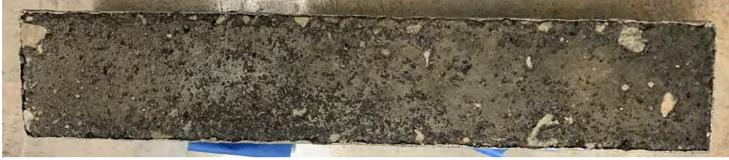
Figure G-3. Mixture 2 after 56 cycles in CDF-A:FT1 testing, average visual rating 2.
