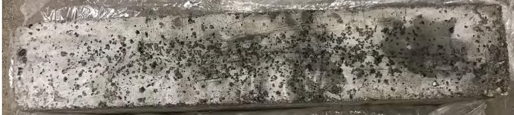
Figure G-13. Mixture 14 (A, NS, N) after 56 cycles in CDF-B:FT4 testing, average visual rating 1.
