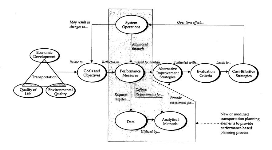
Figure 2. Elements of a performance-based planning process.
