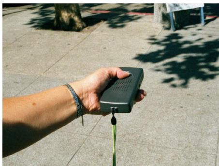
Figure 5. A receiver-based system provides information to a receiver carried by the user.
