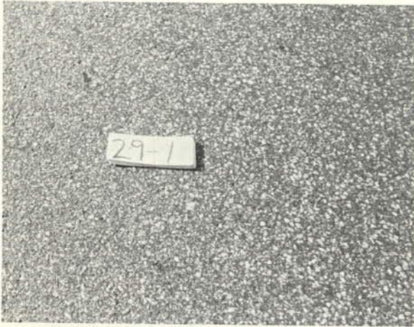
A bituminous mat which is the color of the aggregate between the wheelpaths because the bituminous material has been eroded off of the aggregate and the aggregate does not protrude. (Rating 4.0)
