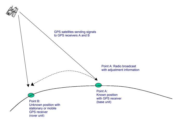
FIGURE 9 Real-time differential correction of GPS signal.
