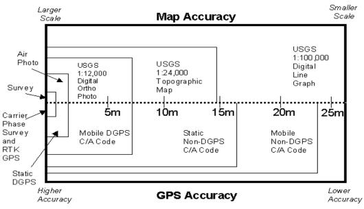
FIGURE 6 GPS and GIS accuracy (at 95 percent confidence interval) (source: Bob Lewis, Navstar Mapping Corp.).
