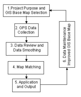
FIGURE 3 GPS-GIS integration process.
