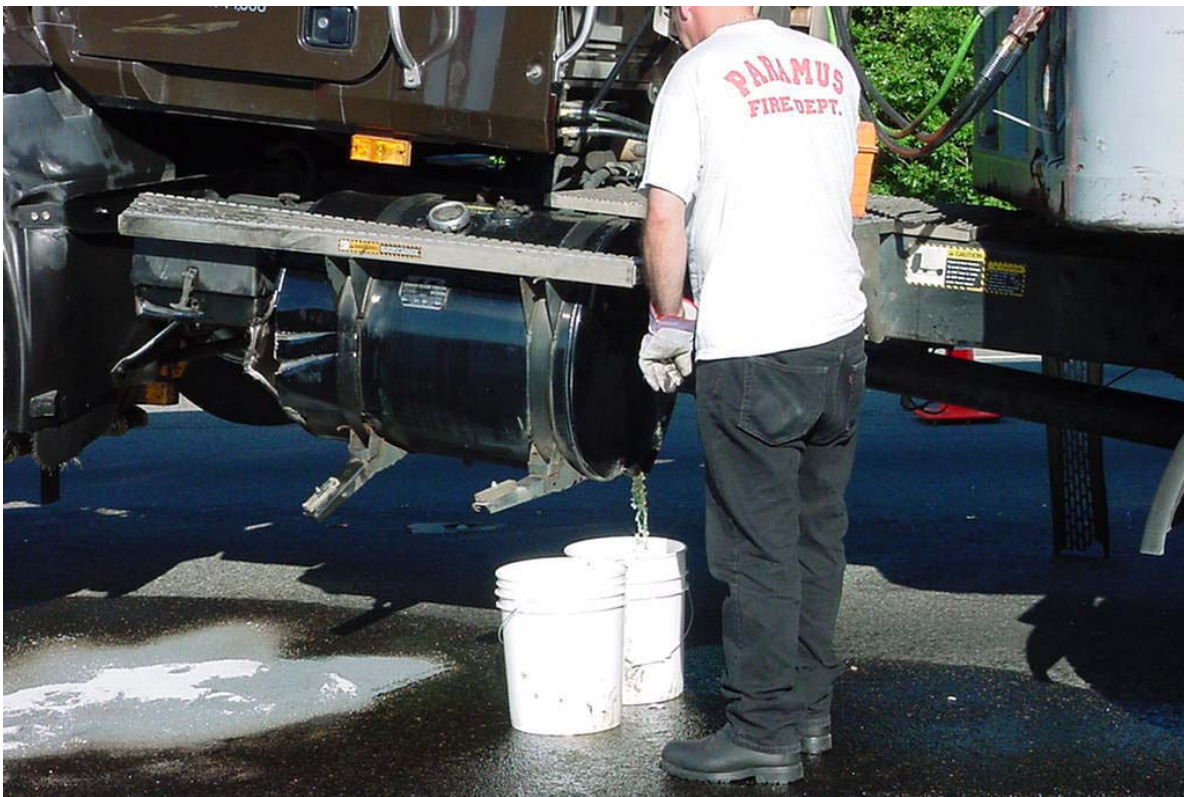
FIGURE 28 The location of truck diesel saddle tanks makes them particularly vulnerable to rupture in a crash. (Courtesy: New Jersey DOT.)
