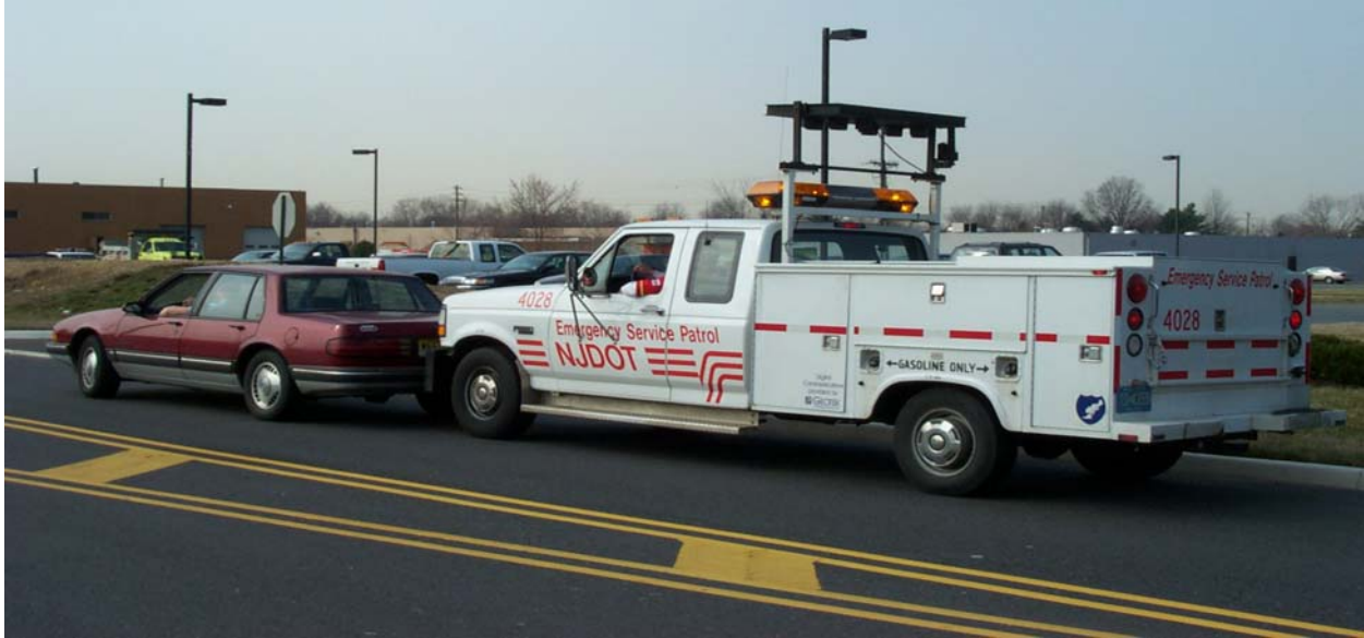
FIGURE 12 New Jersey DOT's Emergency Service Patrol removal of a disabled vehicle from the main traveled way of the road. (Courtesy: New Jersey DOT.)
