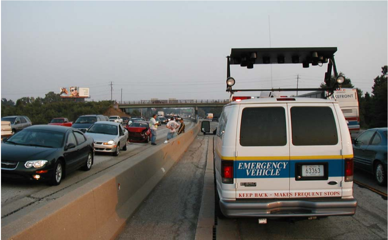
FIGURE 20 Freeway service patrol, parked in the median shoulder, at the scene of a property-damage-only crash blocking the median shoulder.
