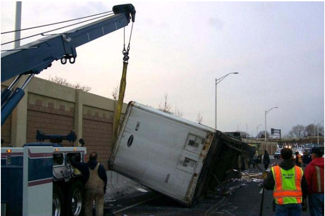
FIGURE 25 Recovery truck with rotator righting an overturned semi-tractor trailer. (Courtesy: New Jersey DOT.)
