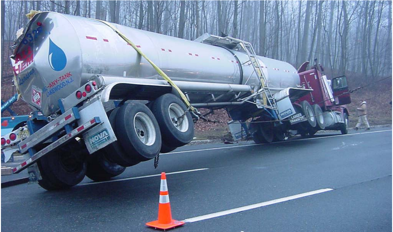
FIGURE 24 Two heavy-duty tow trucks (mostly obscured) in the process of righting an overturned tanker truck. (Courtesy: New Jersey DOT.)
