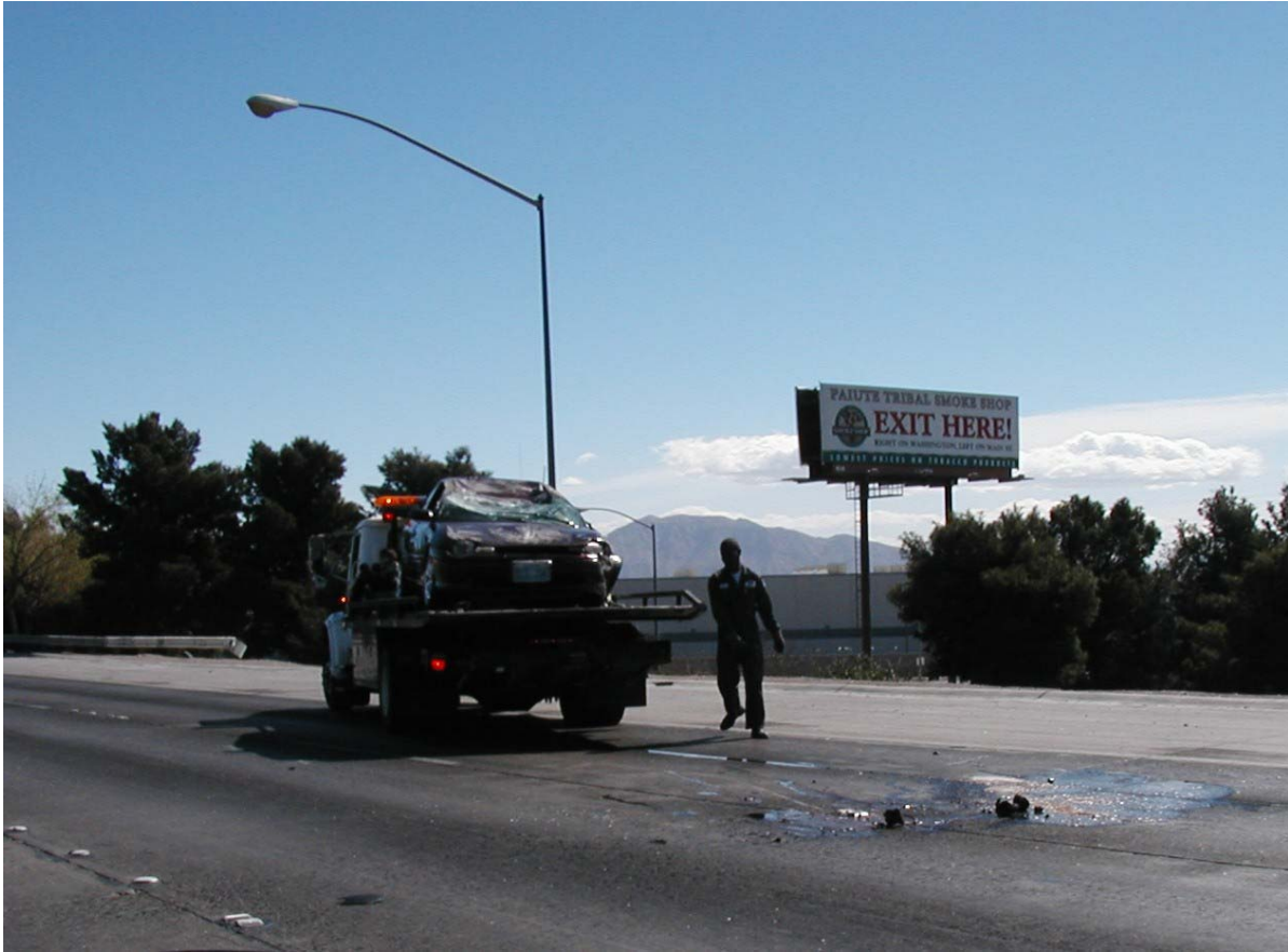
FIGURE 29 The occurrence of incidental vehicle fluid spills can delay the opening of travel lanes if on-scene responders do not have the appropriate training and equipment to identify and remove the hazard.
