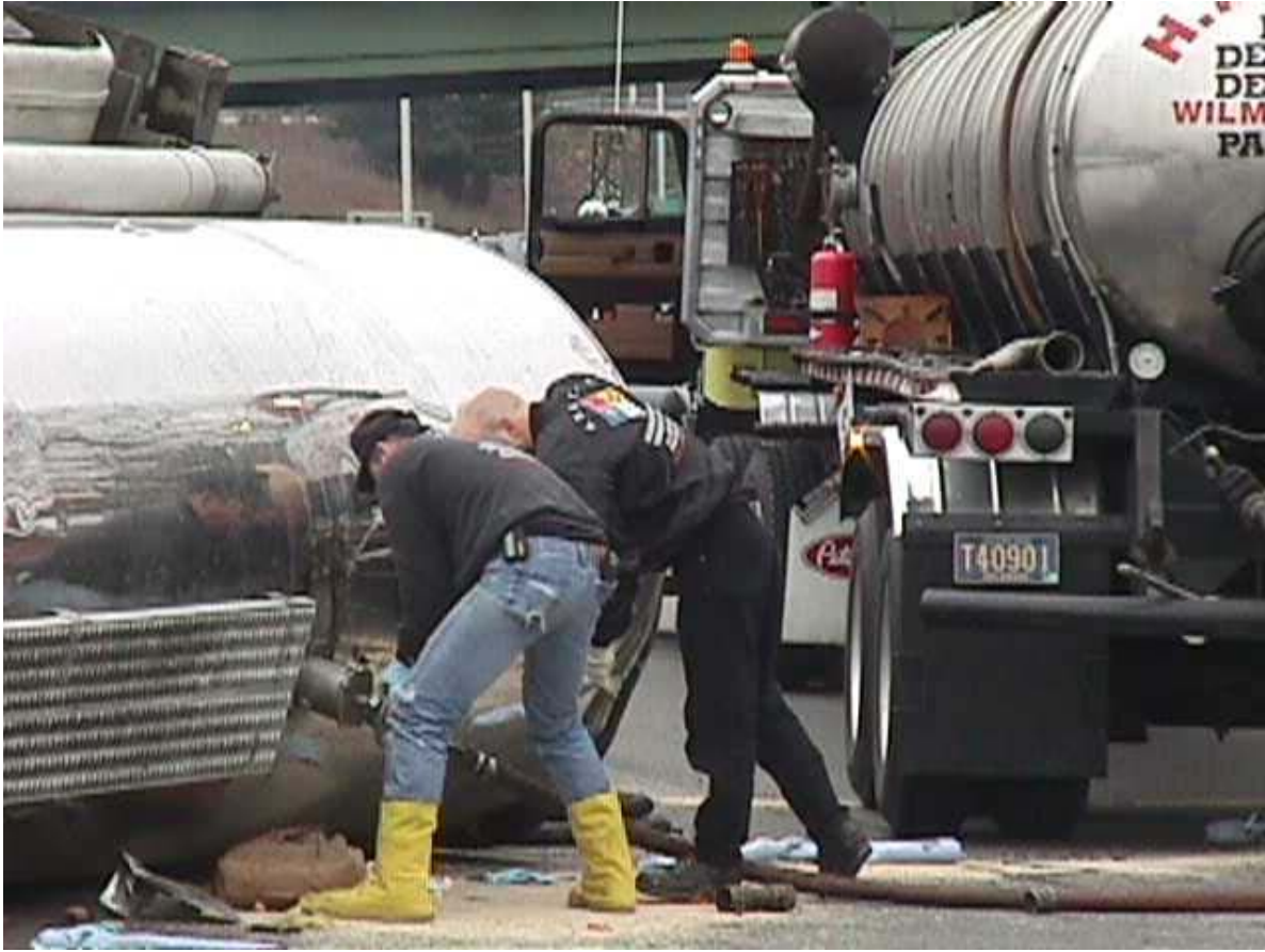
FIGURE 23 Incident responders transferring the contents of an overturned tanker truck to an empty tanker truck before righting the wrecked vehicle. (Courtesy: New Jersey DOT.)
