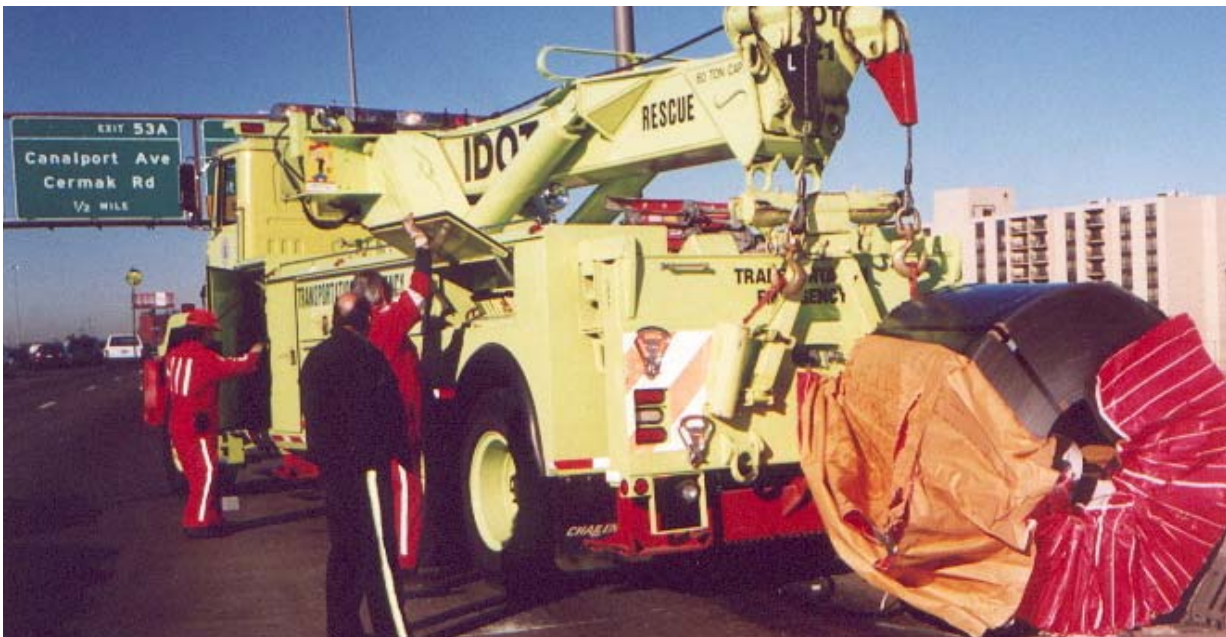
FIGURE 9 Emergency traffic patrol 60-ton-capacity rotator removing spilled cargo from an expressway. (Courtesy: Illinois DOT–District 1.)
