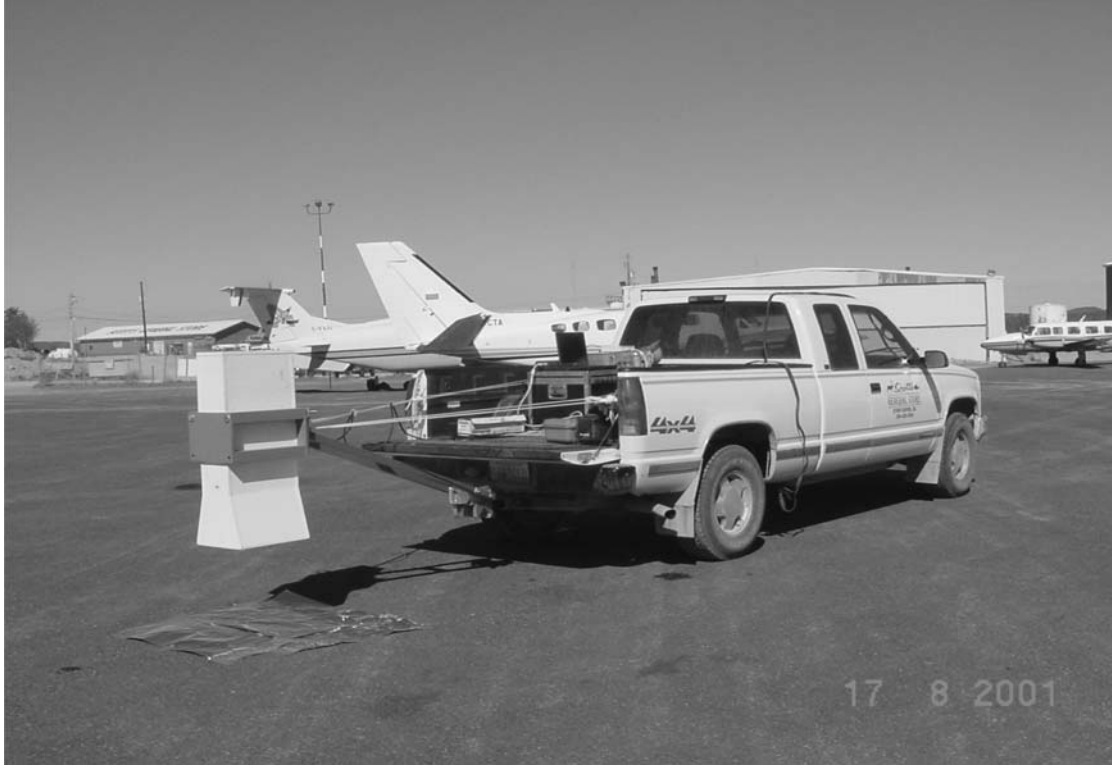
FIGURE D3 Truck-mounted GPR at Stony Rapids Airfield.
