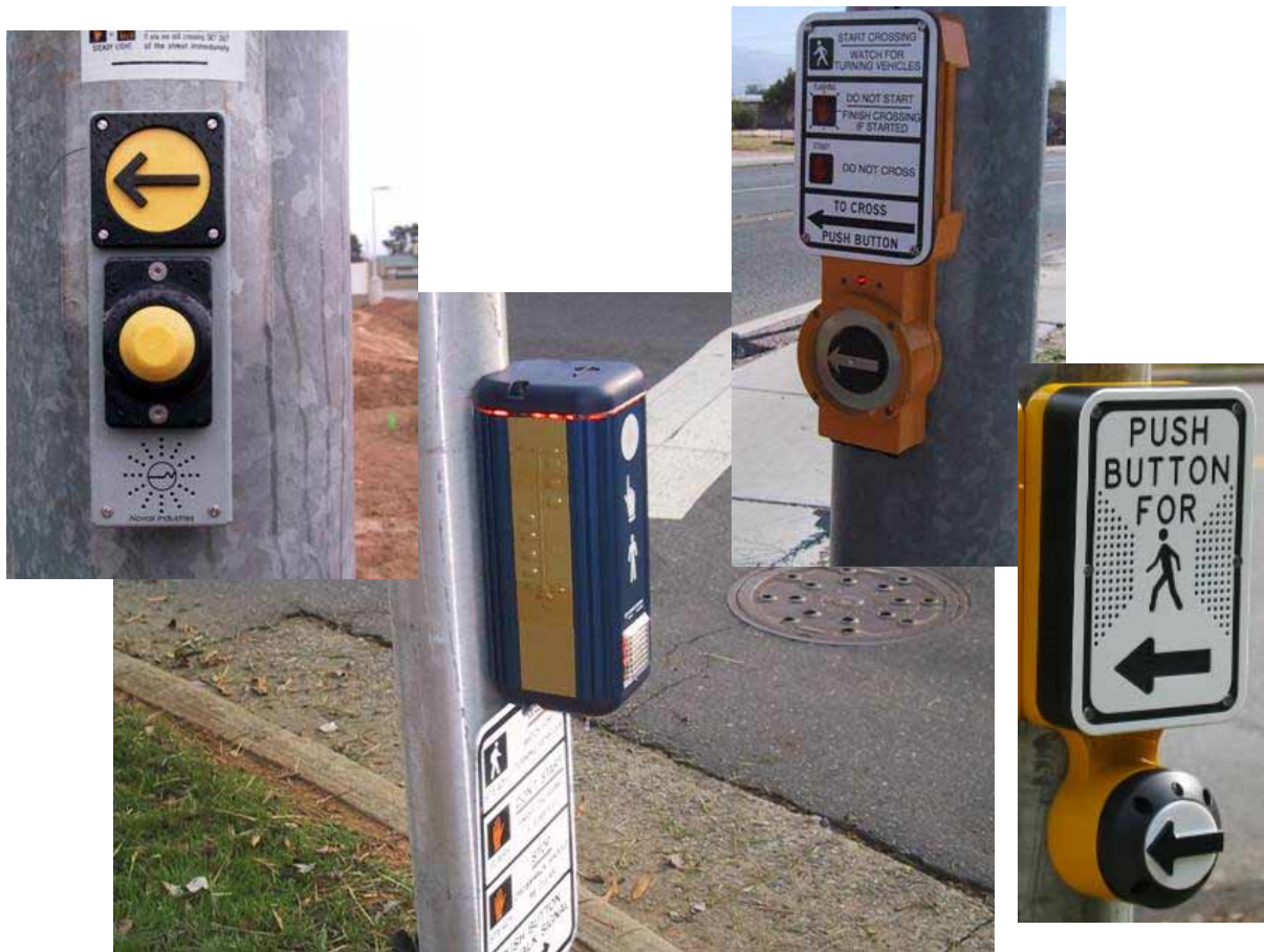
Figure 3-4. Pushbutton-integrated APS units from four manufacturers were deployed for the experiments.
