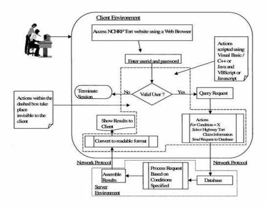
Figure 1.1 Scheme of Client Environment for Web-based Interface
