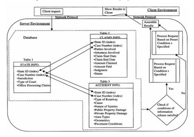
Figure 1.2 Scheme of Server Environment for Data Processing
