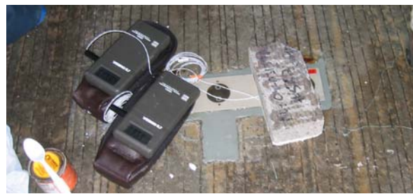
Figure 8. Completed Pavement Temperature Test Setup (Only One Thermistor Required).
