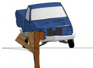
Figure D-3. [CONTINUED] Sequential views from a downstream and overhead viewpoint for analysis case: 47% baseline anchor strength and DL1 posts.
