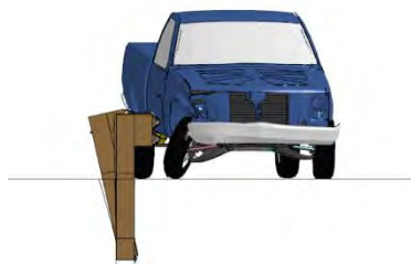
Figure J-4. [CONTINUED] Sequential views from a downstream and overhead viewpoint for analysis case: 35 mph at Impact Point 2.
