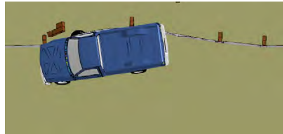
Figure M-1: [CONTINUED] Sequential views from a downstream and overhead viewpoint for 6-inch erosion a single post analysis case.
