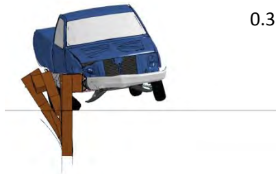
Figure M-1: [CONTINUED] Sequential views from a downstream and overhead viewpoint for 6-inch erosion a single post analysis case.
