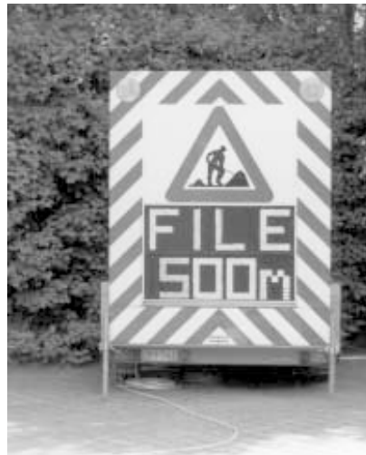
Figure 3. Trailer-mounted variable message signs are linked to video cameras in Belgium; as traffic slowdowns are detected, a warning is posted on the sign.
