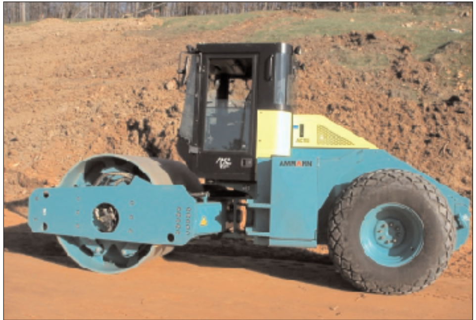
The Amman Compaction Expert (ACE) for intelligent soil compaction.
