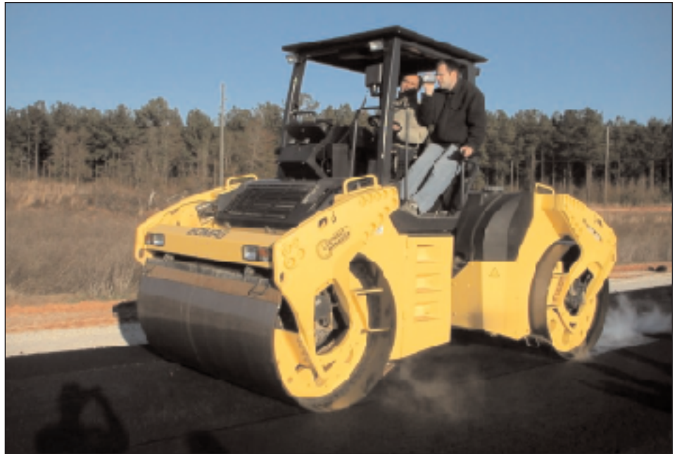
Bomag Asphalt Manager for hot mix intelligent compaction.
