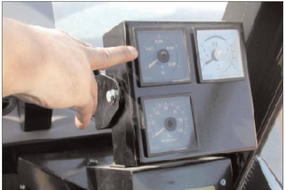
The roller operator's console with O.K. zone clearly marked.
