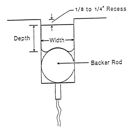
Figure 1. Cross section of a concrete joint sealed with a field-cured sealant.
