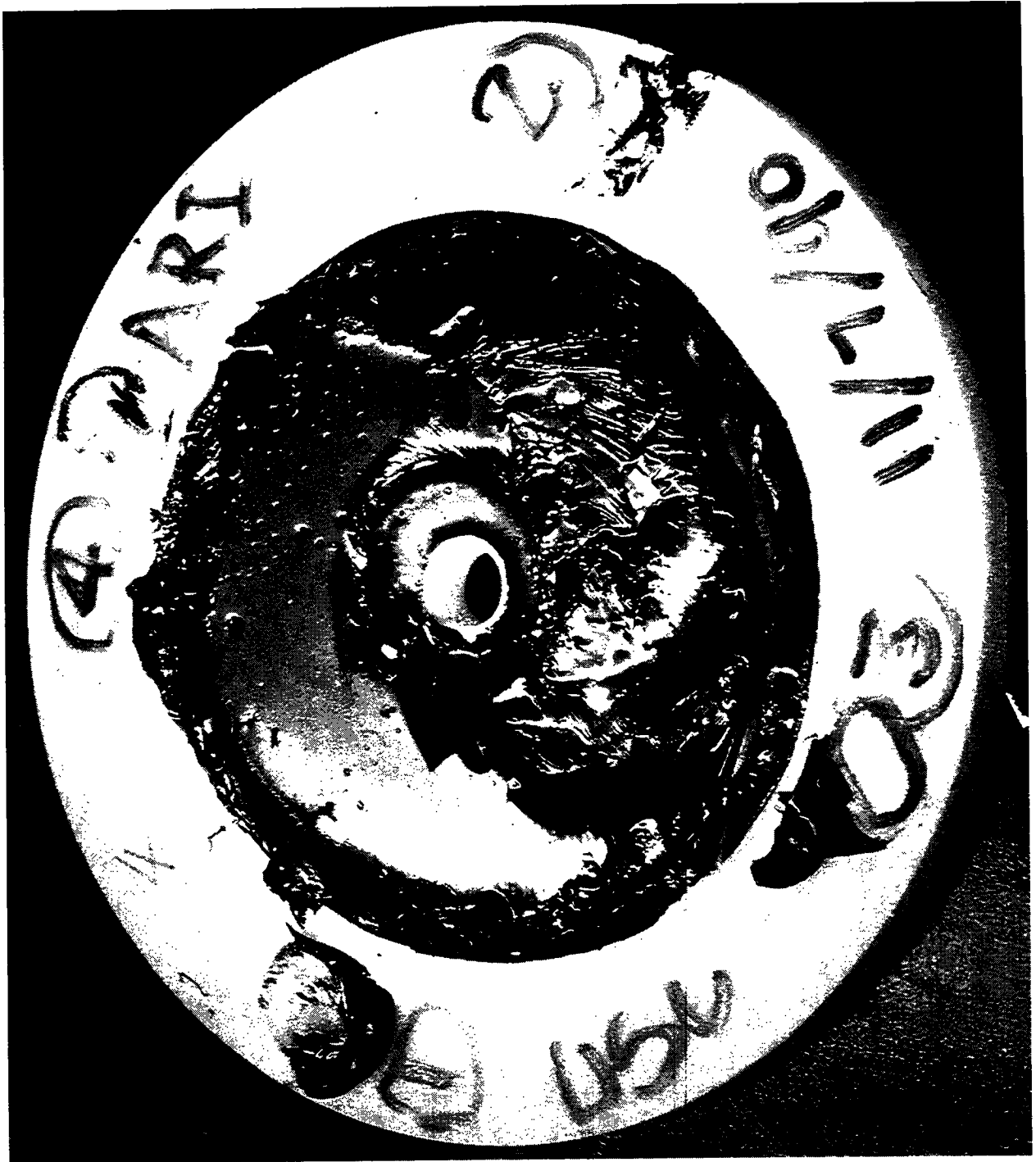
Figure 7.6: The blister test fracture surface of modified specimen of Teflon-AAK system, with failure taking place in the bulk asphalt.
