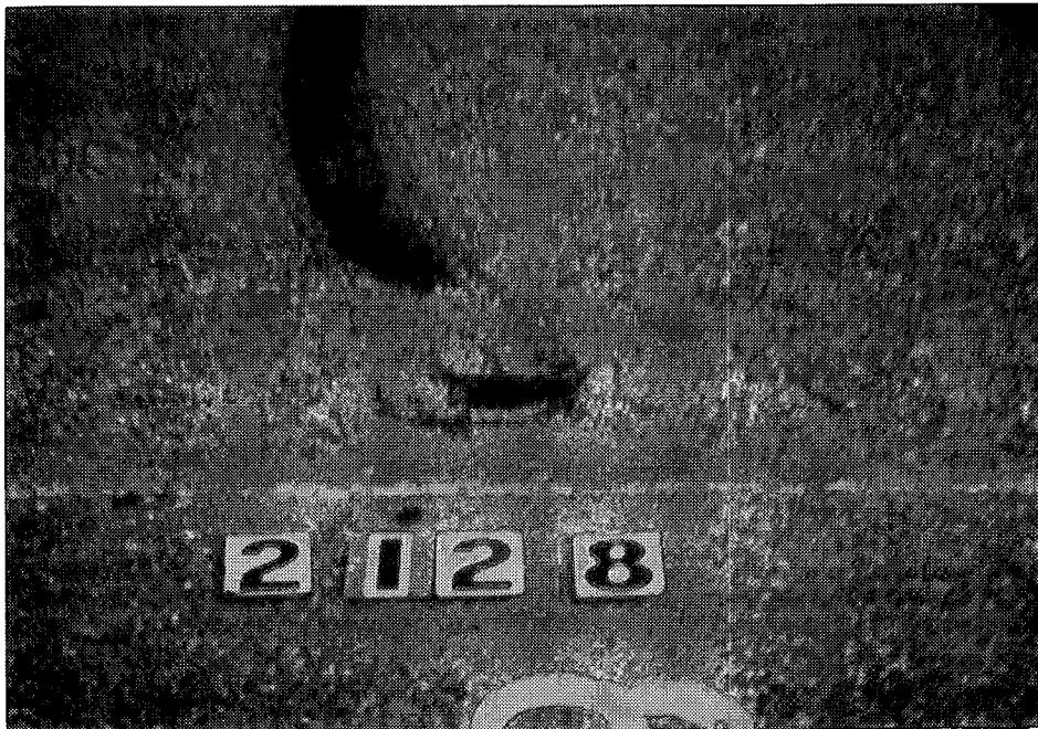
Figure 29. High-severity pull-out of Koch 9030 band-aid seal at Abilene
