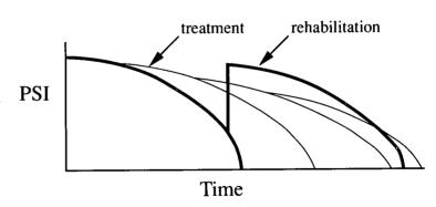
as shown by the light lines in the figure above. Thus, applying modest-cost surface treatments at the right time can delay the need for future major rehabilitation. This will save money in the paving budget. It may also save in the high cost of longer traffic delays and increased accidents that major reconstruction work zones often produce.
