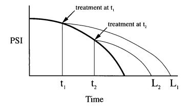
The initial data from observing the test sections started in SHRP H-101 also suggest that the pavement life will be extended longer if a particular maintenance treatment is applied before significant deterioration has set in, rather than waiting until the pavement has deteriorated badly. The figure to the left shows the type of increased life the initial research suggests that early surface treatment will provide as compared to applying the maintenance treatment later.
