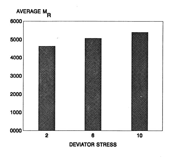
Figure 5. Average  $M_R$  by Deviator Stress for Synthetic Specimen DPTU-1560.
