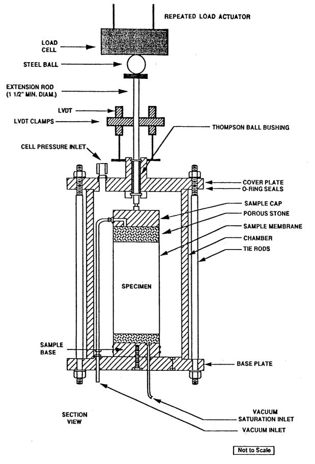
Figure 1. Triaxial chamber with external LVDT's and load cell.
