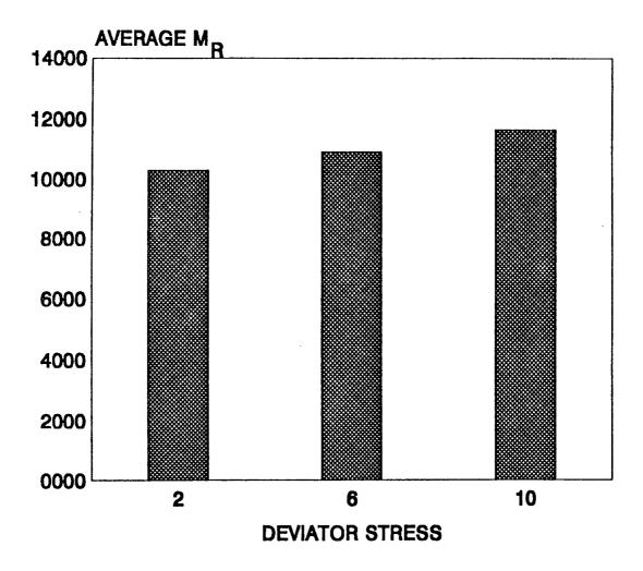
Figure 6. Average  $M_R$  by Deviator Stress for Synthetic Specimen TU-960.
