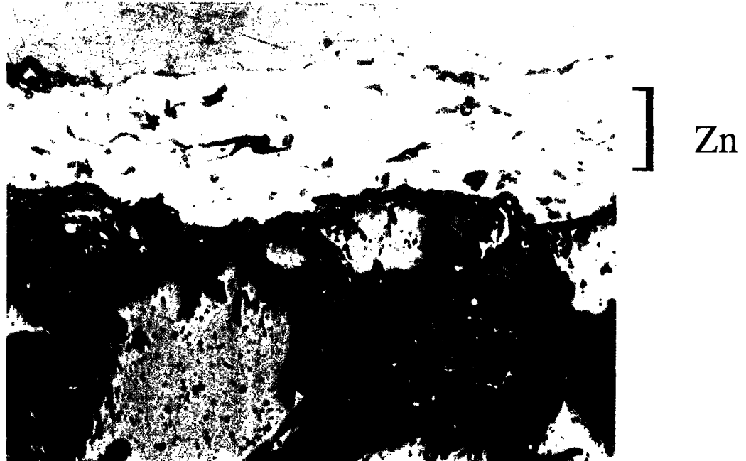
Figure 4.12 Typical microstructure of arc-sprayed zinc as revealed in a metallographic cross section. The dark regions and thin lines are porosity resulting from impact and solidification of consecutive droplets on the sprayed surface. Notice how the deposited zinc closely follows the concrete surface. Cement paste and fine aggregates are visible. The coating on this specimen was approximately 250 \mu\text{m} thick. The field shown is 900 \mu\text{m} from top to bottom.
