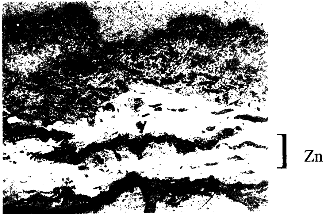
Figure 4.13 Microstructure of a zinc deposit after approximately 200 days of galvanic service in the 85% relative humidity environment. Porous deposits are present on the outer (top) surface. Zinc corrosion has taken place at the porous pockets between zinc layers and, to a lesser extent, between the zinc and the concrete. The concrete matrix is at bottom. The field shown is 900 \mu\text{m} from top to bottom.
