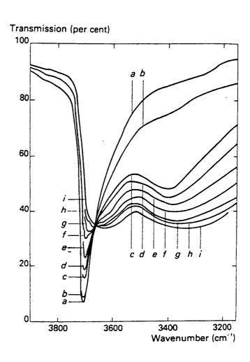
Figure 4. Infrared spectra of silica immersed in (a) heptane, (b)-(i) solutions in heptane of N, N-diethylaniline at concentrations (mmol dm³) of 1 · 4, 4 · 1, 5 · 5, 11,28, 41, 69 and 138 respectively
