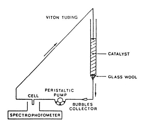
Figure 3. Continuous Adsorption Apparatus
