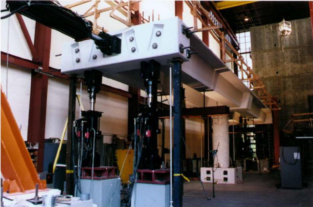
Figure 67. Type of specimen investigated -- note the detail over the pier. Steel bridge system with integral pier
