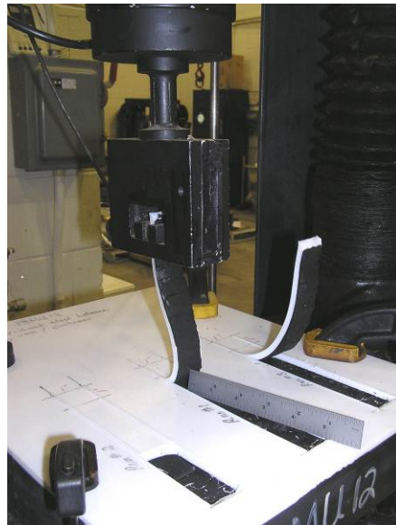
Figure 18. Bearing testing. Source: NYSDOT.
