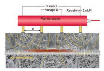
Figure 3.17. Electrical resistivity principle.
