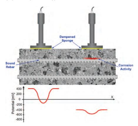
Figure 3.15. GPM principle.
