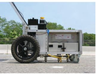
Figure 3.5. USW testing using a portable seismic property analyzer (PSPA).
