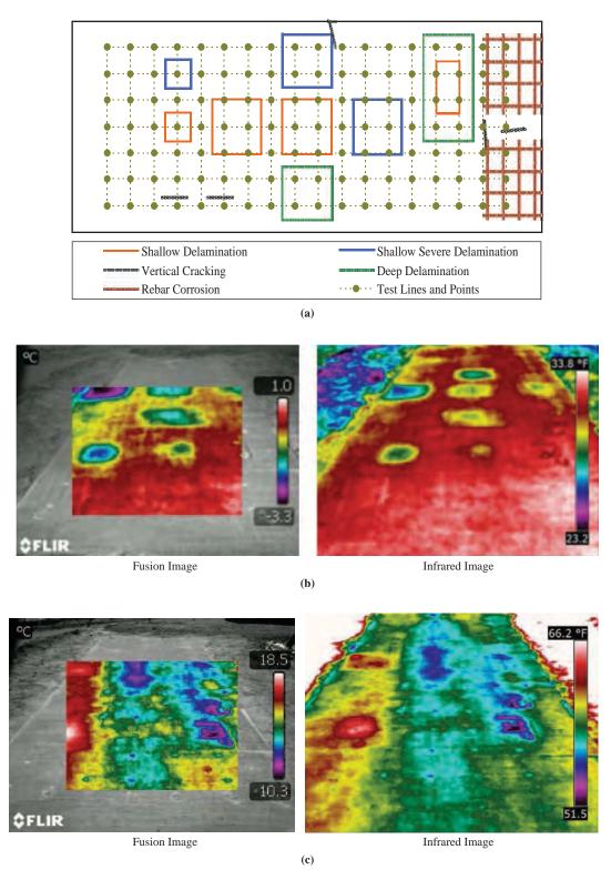
Figure 6.11. Infrared images: plan of fabricated deck (a) and Participant 2 (b, c). Infrared image (c) is taken from the opposite side.
