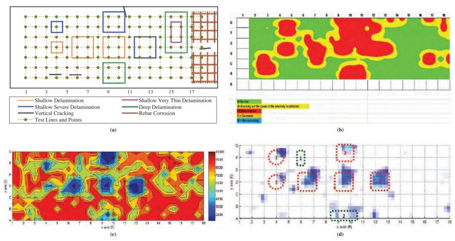
Figure 6.7. Impact echo condition maps: plan of fabricated deck (a), Participant 4 (b), and Participant 6 (c, d).
