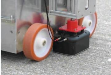
Figure 3.3. Shear-wave probe array A1220 (left), and automated A1220 measurements using stepper (right).
