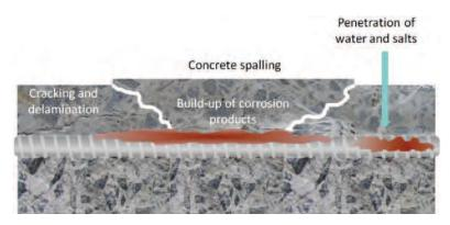
Figure 2.2. Corrosion process.
