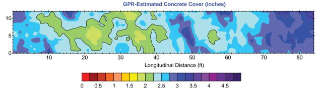
Figure 6.4. Concrete cover estimation based on GPR results.
