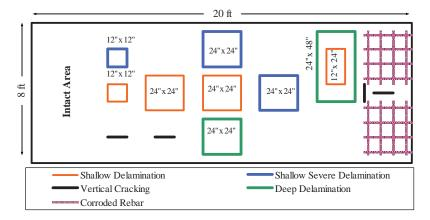
Figure 5.15. Overview of defect distributions in fabricated slab.
