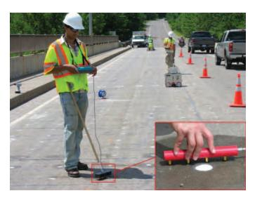
Figure 3.16. Electrical resistivity testing using a Wenner probe.
