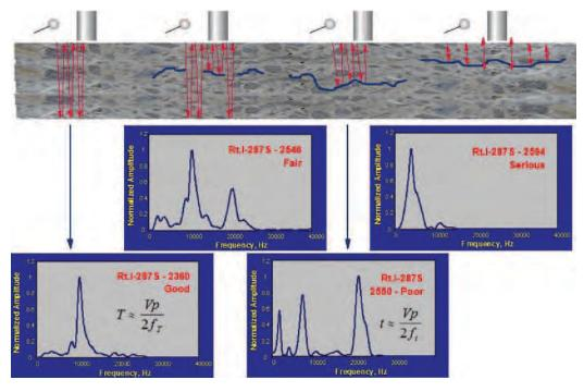
Figure 3.2. Grades for various degrees of deck delamination.
