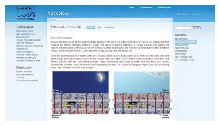
Figure 8.3. Physical principle of infrared thermography.
