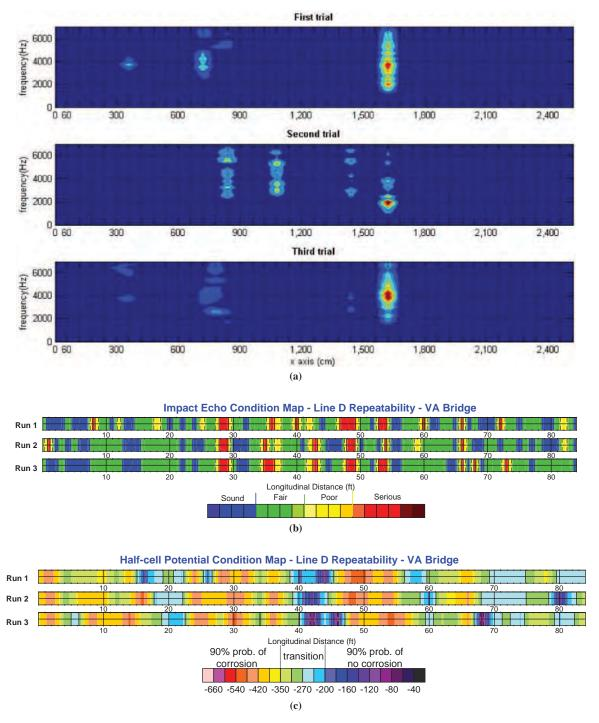
Figure 6.6. Repeatability measurement results. Spectral amplitude, air-coupled IE (a); ratings based on spectral frequency, IE (b); voltage, HCP (c).
