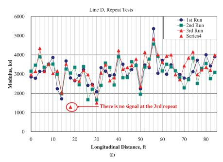
Figure 6.6. (continued) Repeatability measurement results. Resistivity, ER (d); signal attenuation, GPR (e); and modulus, USW (f).
