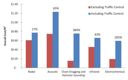
Figure 7.5. The overall cost of survey (with and without traffic control).
