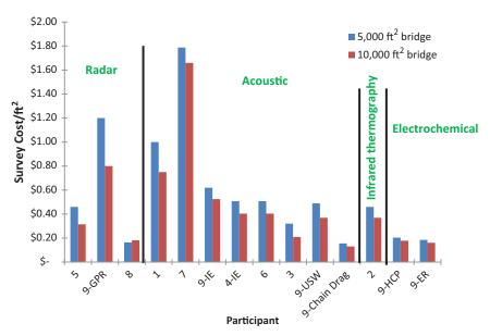
Figure 7.2. Cost per square foot for the assumed surveys on 5,000-ft<sup>2</sup> and 10,000-ft<sup>2</sup> bridge decks (excluding traffic control).
