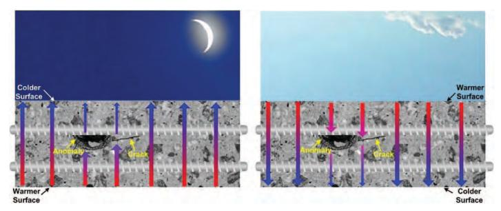
Figure 3.20. Principle of passive infrared thermography.
