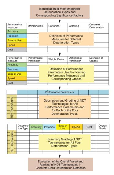
Figure 4.1. Flowchart of the categorization and ranking process of NDT technologies.
