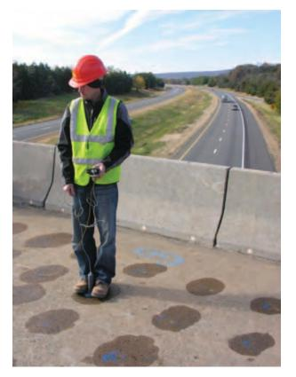
Figure 5.10. Impact echo and surface waves (left) and galvanostatic pulse measurement (right): Olson Engineering.
