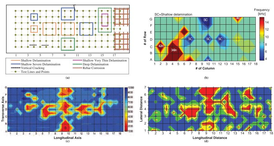
Figure 6.8. Impact echo condition maps: plan of fabricated deck (a), Participant 7 (b), Participant 10 (c), and Participant 9 (d).
