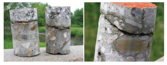
Figure 2.4. Delamination observed in extracted cores.
