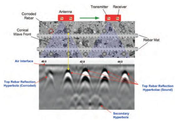
Figure 3.11. GPR principle.
