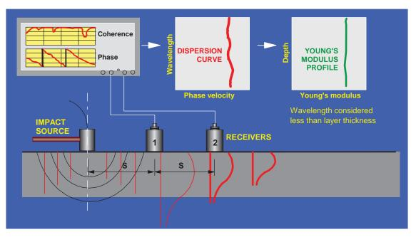
Figure 3.7. Schematic of surface wave velocity versus wavelength (top) and evaluation of a layer modulus by SASW (USW) method (bottom).
