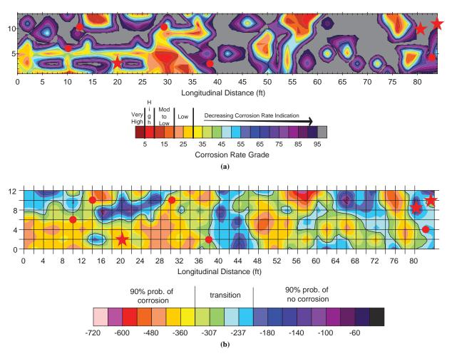
Figure 6.5. Electrical resistivity (a) and HCP (b).
