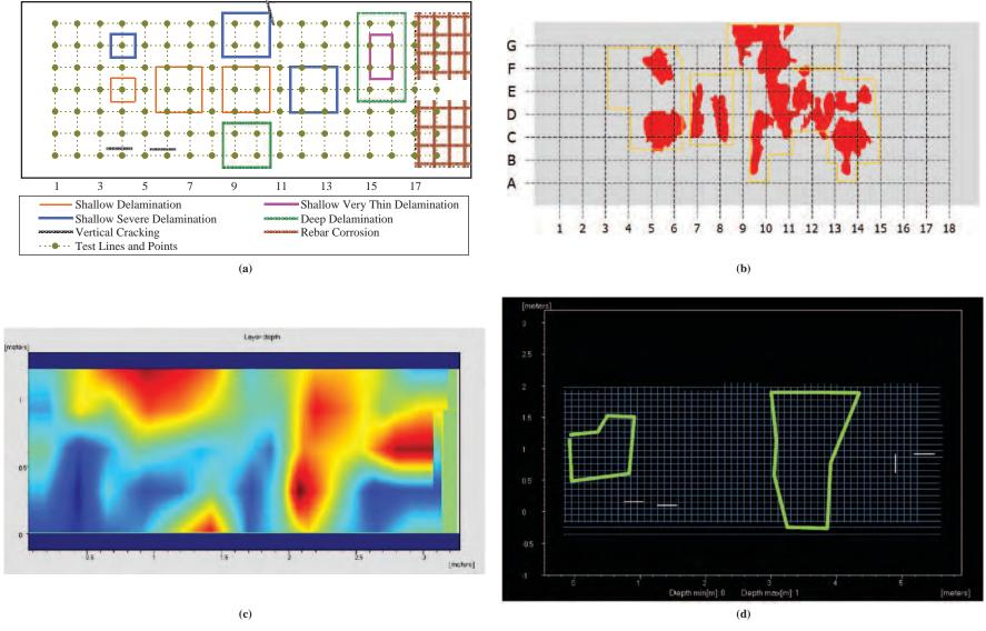
Figure 6.9. GPR condition maps: plan of fabricated deck (a), Participant 8 (b), Participant 4 (c), and Participant 5 (d).
