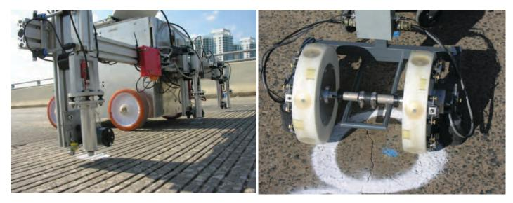
Figure 3.1. Stepper (left) and bridge deck scanner (right).
