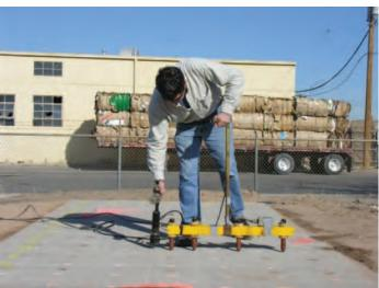
Figure 5.22. Air-coupled impact echo (left): University of Illinois. Impact echo (right): NDT Corporation.
