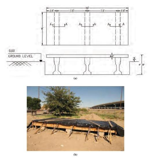
Figure 5.14. Fabricated slab: (a) schematic and (b) curing.
