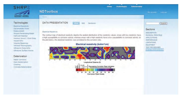
Figure 8.4. Data presentation: Electrical resistivity.
