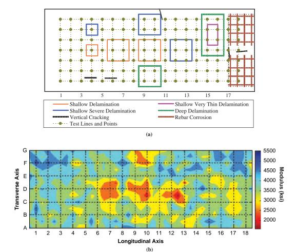
Figure 6.13. Plan of fabricated deck (a) and apparent modulus mapping for delamination (b). Participant 10.
