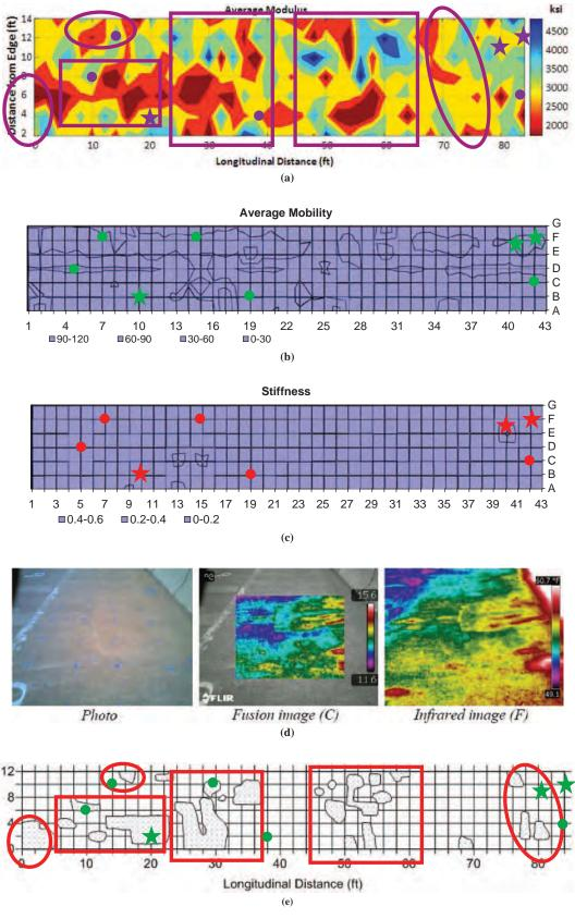
Figure 6.2. USW (a), impulse response (b, c), infrared thermography (d), chain dragging and hammer sounding (e).
