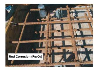
Figure 5.16. Setup of the corroded steel bar mat in the fabricated deck.
