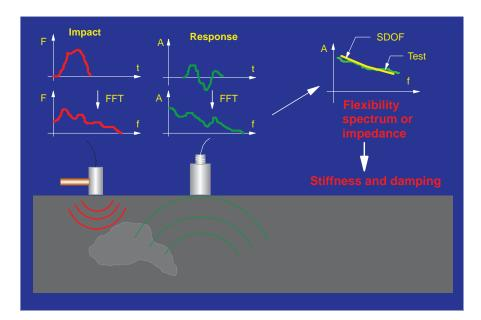
Figure 3.9. Principle of impulse response testing.
