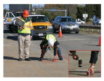
Figure 3.8. Impulse response testing.
