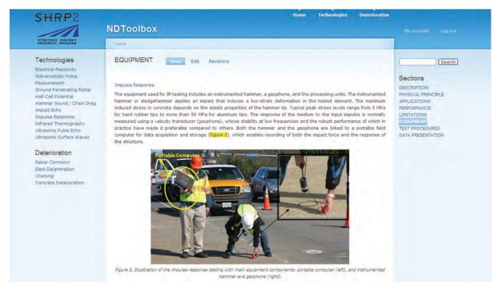
Figure 8.5. Equipment: Impulse response.
