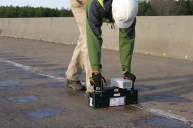
Figure 3.4. Bridge deck survey using MIRA ultrasonic system. B-scans (top) and equipment and data collection (bottom).
