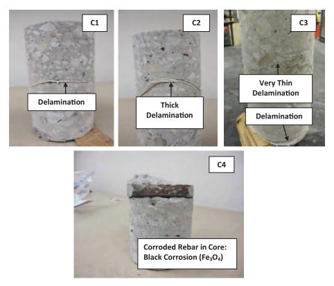
Figure 5.18. Cores from fabricated bridge deck.
