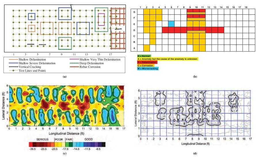
Figure 6.10. GPR condition maps: plan of fabricated deck (a), Participant 1 (b), and Participant 9 (c, d).
