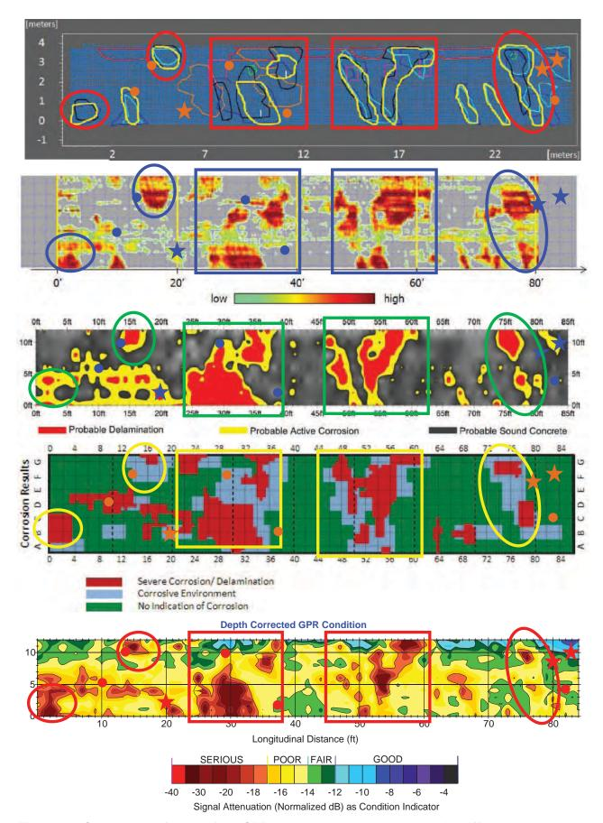
Figure 6.3. Comparison of results from GPR tests on actual bridge section by different participants.
