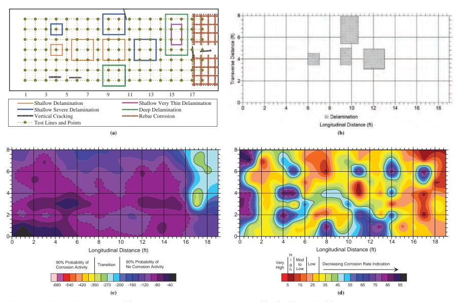
Figure 6.12. Plan of fabricated deck (a), chain dragging and hammer sounding (b), HCP (c), and ER (d). Participant 9.
