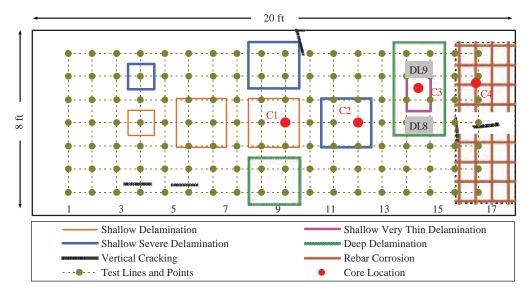
Figure 5.17. Locations of coring on fabricated deck.
