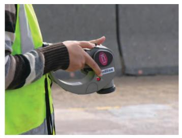
Figure 3.18. Infrared thermography testing.
