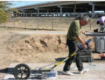
Figure 5.24. Air-coupled impact echo (left): University of Texas at Austin. Ground-penetrating radar (right): Rutgers University.
